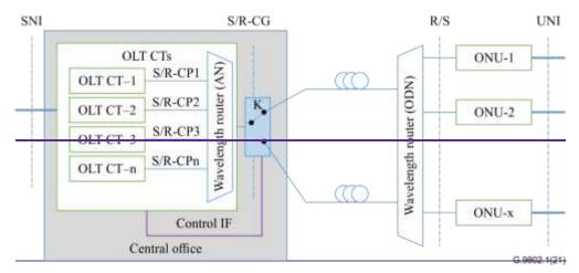
Figure 11-3 – Example of feeder protection through single OLT through an external optical switch
