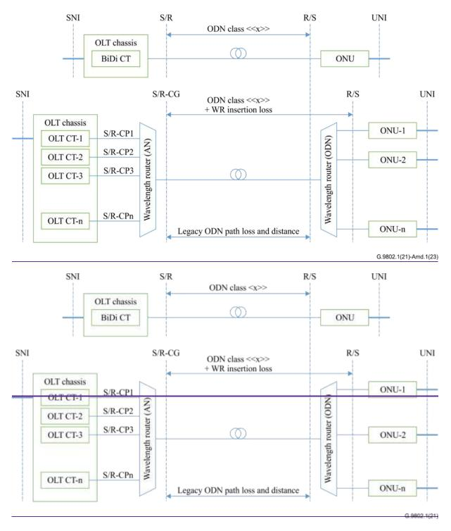
Figure 6-2 – Upgrade example of a legacy link (at the top) to a multi-channel one (bottom)
