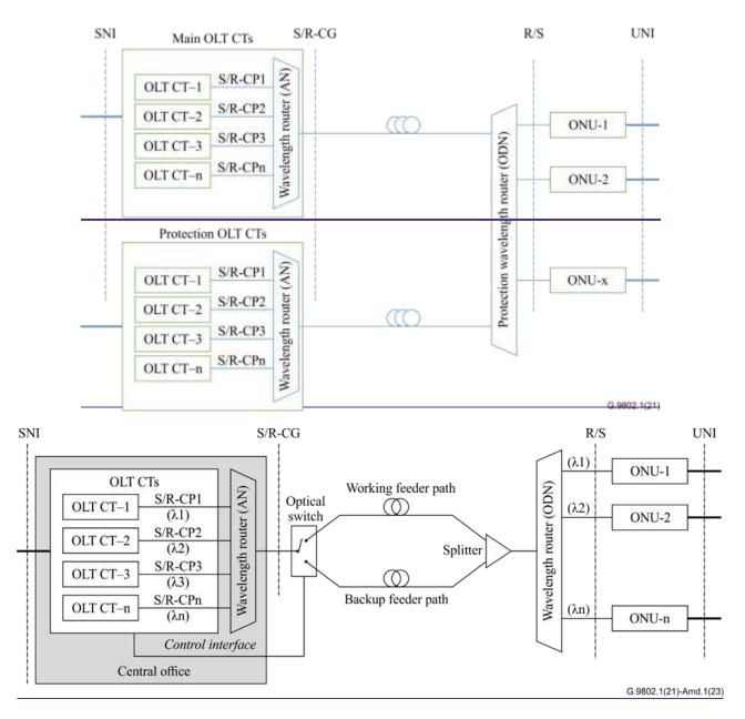
Figure 11–5 – Example of feeder protection through single OLT with an external optical switch
