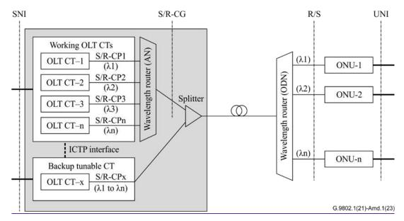
Figure 11–3 – Example of individual CT protection through a splitter and a tunable CT
