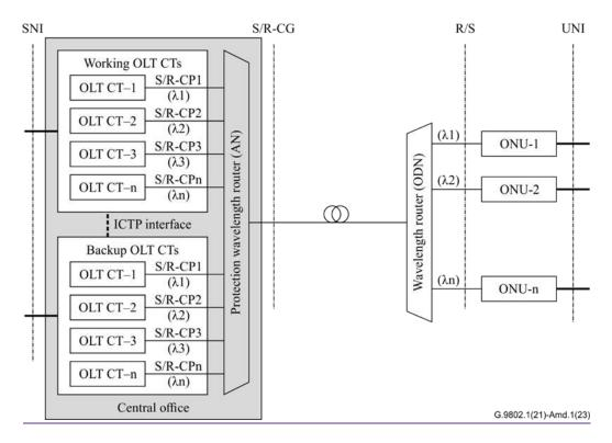
Figure 11–1 – Example of full CT protection scenario
