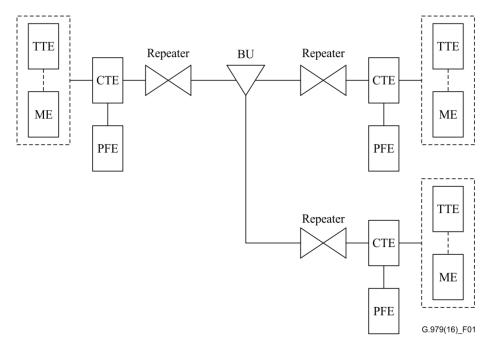
Figure 1 – General architecture of repeatered system
