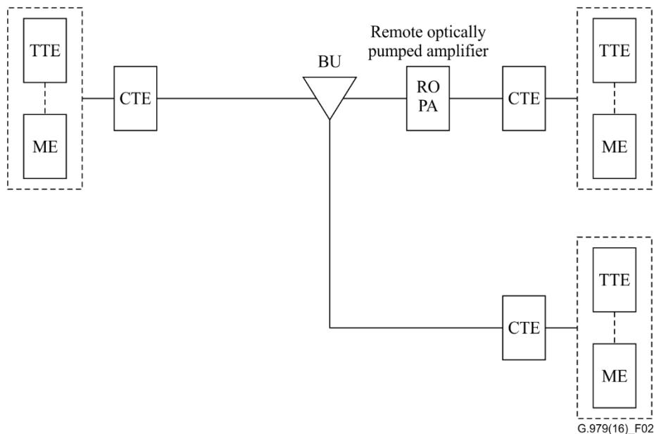
**Figure 2 – General architecture of repeaterless system**
