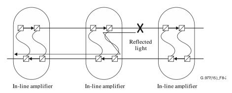
Figure 8-2 – Example of fault location in the first fibre using COTDR for OFA systems using output-to-input coupler
