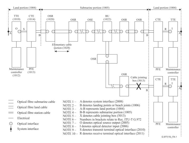
Figure A.1 – Example of repeatered optical fibre submarine cable system
