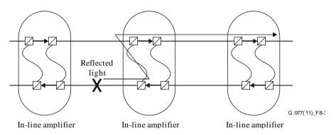
Figure 8-3 – Example of fault location in the second fibre using COTDR for OFA systems using output-to-input coupler
