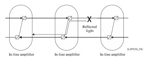
Figure 8-1 – Example of fault location using COTDR for OFA with output-to-output loopback coupling
