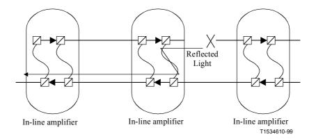
Figure 5/G.977 – Example of fault location using COTDR for OFA systems using output-to-input coupler
