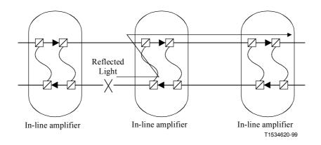
Figure 6/G.977 – Example of fault location using COTDR for OFA systems using output-to-input coupler
