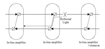
Figure 4/G.977 – Example of fault location using COTDR for OFA with output-to-output loopback coupling
