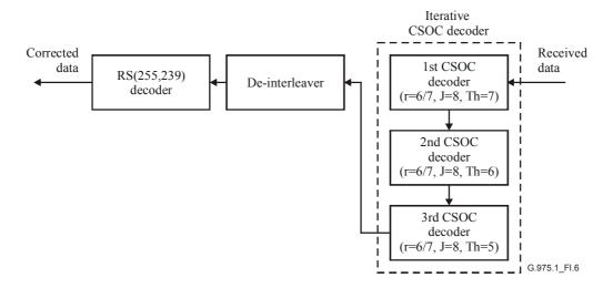
Figure I.6/G.975.1 – An example of the super-FEC decoder
