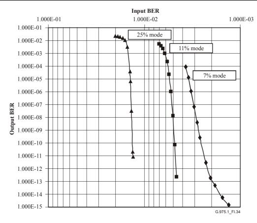
Figure I.34/G.975.1 – FEC performance input BER vs output BER
