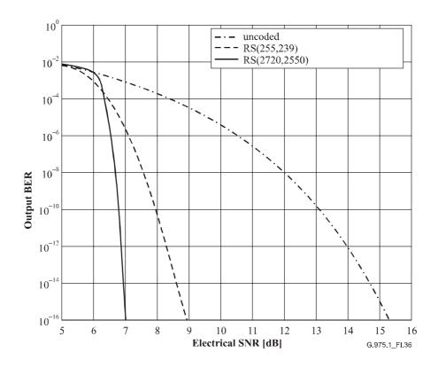
Figure I.36/G.975.1 – Output BER as a function of the input  $E_b/N_\theta$  for the RS(2720,2550) code and the standard FEC code
