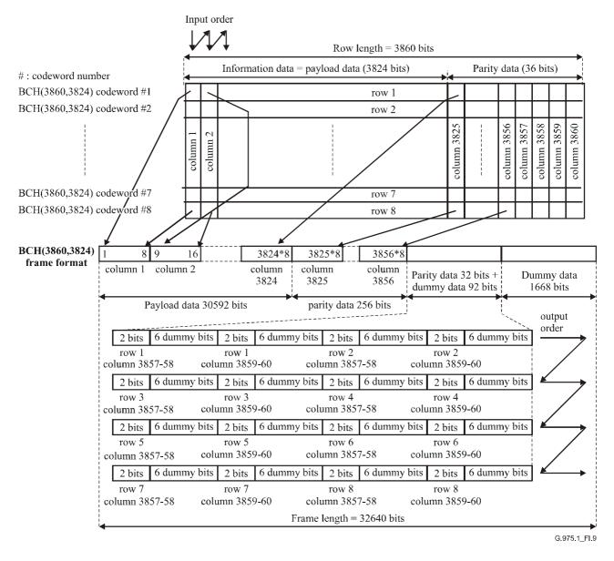
Figure I.9/G.975.1 – BCH(3860,3824) frame format
