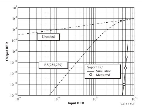
Figure I.7/G.975.1 – BER characteristics of the super-FEC decoder
