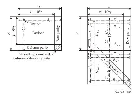
Figure I.21/G.975.1 – Concept of orthogonally interleaved codewords as matrix or streaming structure
