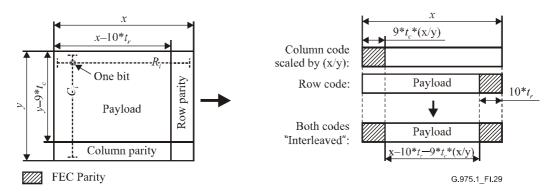
Figure I.29/G.975.1 – Simplification of interleave to support rate computation
