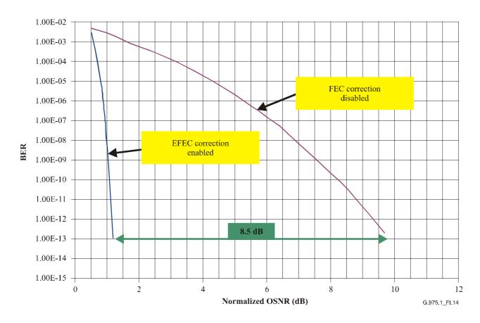
Figure I.14/G.975.1 – Net coding gain
