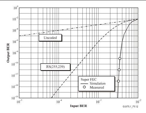
Figure I.12/G.975.1 – BER characteristics of the super-FEC decoder
