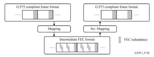
Figure I.20/G.975.1 – Basic remapping scheme
