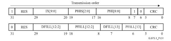
Figure I.31/G.975.1 – Structure of the mapping synchronization pattern
