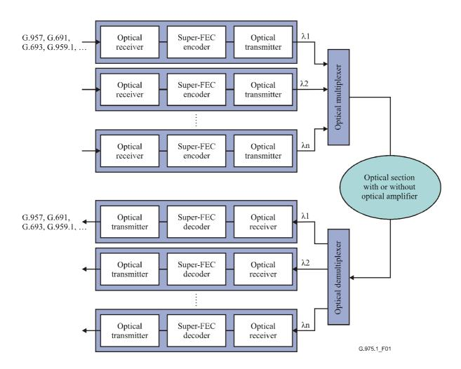
Figure 1/G.975.1 – Block diagram of DWDM submarine optical fibre system
