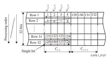
Figure I.27/G.975.1 – Basic mapping to internal framing
