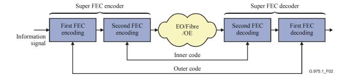
Figure 2/G.975.1 – Outer code and inner code
