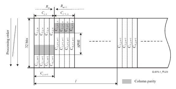
Figure I.23/G.975.1 – General mapping of column codewords over the data stream
