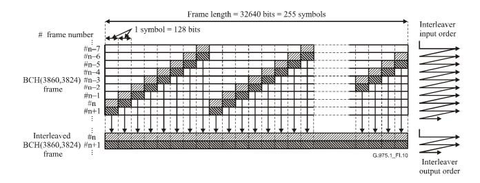
Figure I.10/G.975.1 – Interleaved BCH(3860,3824) frame format
