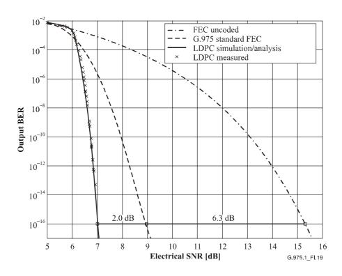
Figure I.19/G.975.1 – Output BER as a function of the electrical SNR for the LDPC code and the existing standard RS FEC code
