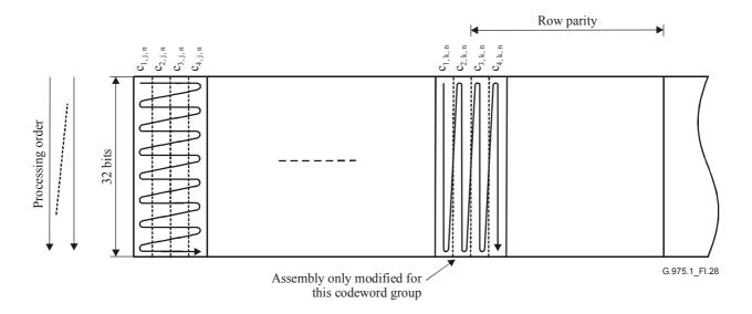
Figure I.28/G.975.1 – Mapping for the 25% mode
