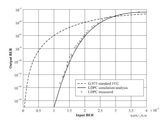
Figure I.18/G.975.1 – Output BER as a function of the input BER for the LDPC code and for comparison with the G.975 standard RS FEC code
