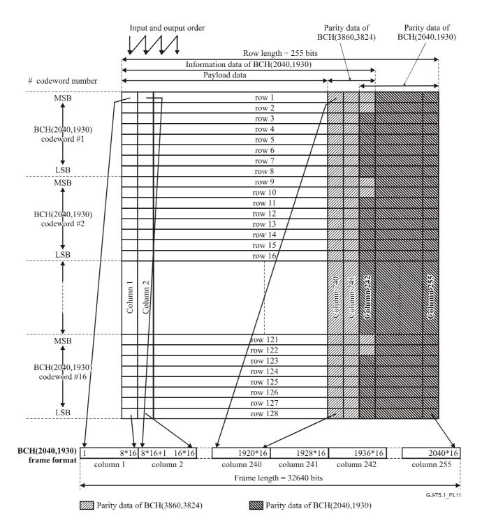
Figure I.11/G.975.1 – BCH(2040,1930) frame format
