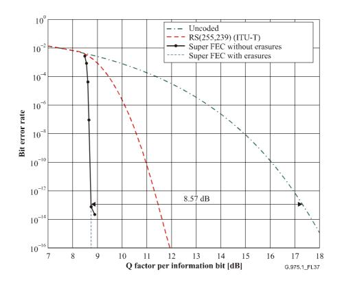
Figure I.37/G.975.1 – Coding gain
