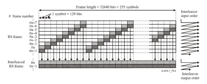
Figure I.4/G.975.1 – Interleaved RS frame format
