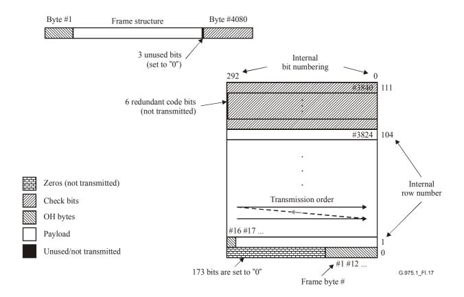
Figure I.17/G.975.1 – Mapping structure for the LDPC code
