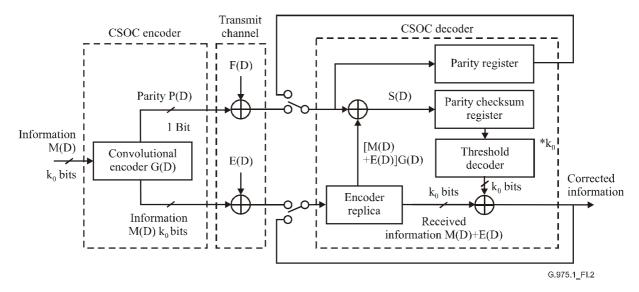
Figure I.2/G.975.1 - CSOCs encoder and decoder
