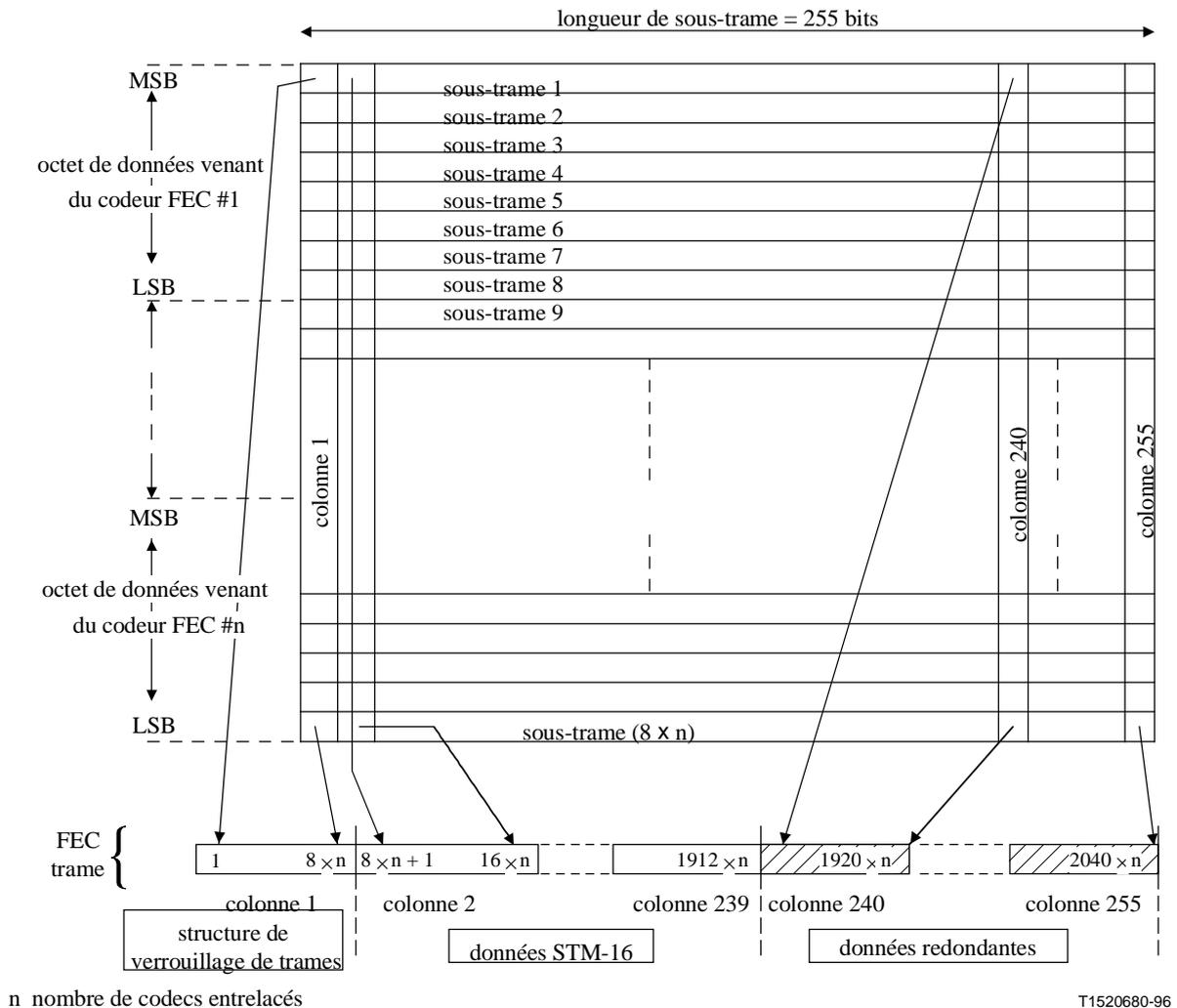
**Figure 4/G.975 – Construction de la trame FEC**
