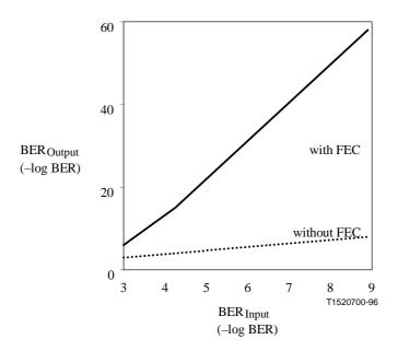
Figure 6/G.975 – Theoretical output versus input BER
