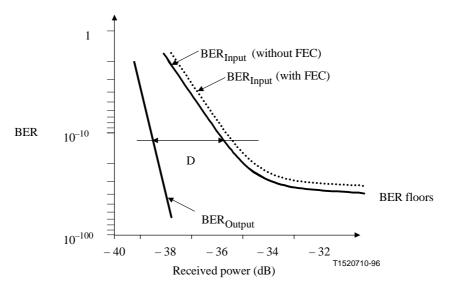
Figure 7/G.975 – Coding gain (D) evaluation scheme
