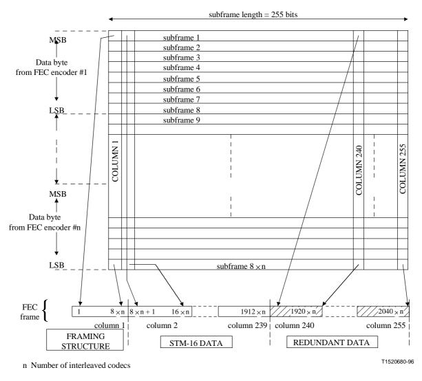
Figure 4/G.975 – FEC frame construction
