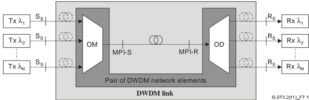
**Figure 7-1 – "black-link" approach for unidirectional applications**
