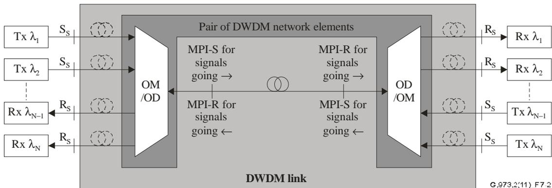
**Figure 7-2 – "black-link" approach for bidirectional applications**
