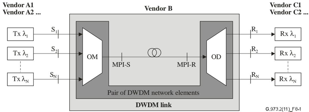
**Figure 8-1 – Single-span black-link transverse compatibility**
