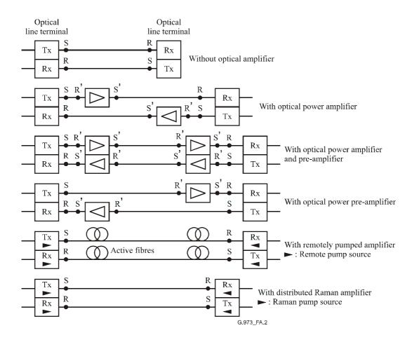
Figure A.2 – Possible system configurations
