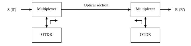
Figure B.2 – Example of line monitoring using OTDR
