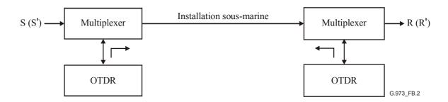
Figure B.2/G.973 – Example of line monitoring using OTDR
