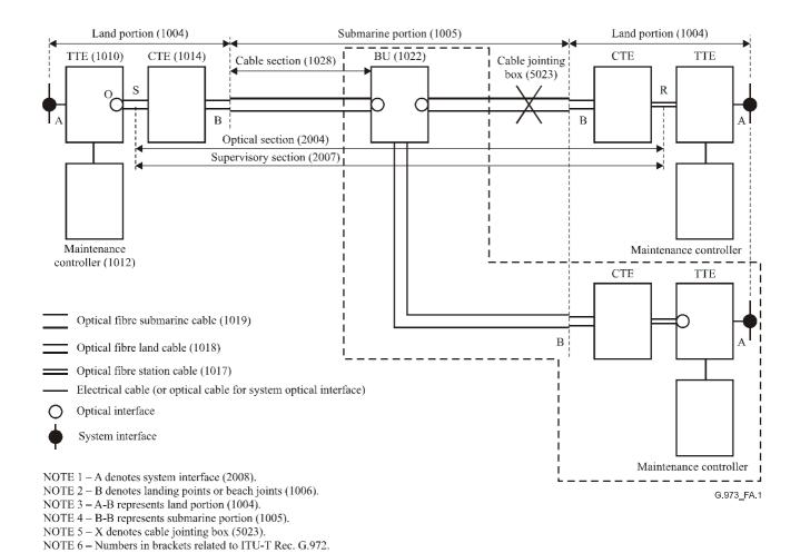
Figure A.1/G.973 – Example of repeaterless optical fibre submarine cable system
