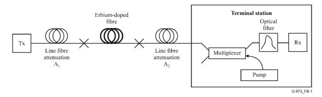
Figure B.1/G.973 – Example of system configuration with remotely pumped optical amplifier from the receiver end
