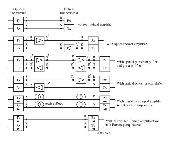
Figure A.2/G.973 – Possible system configurations
