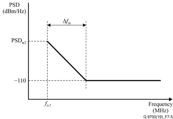
**Figure 7-5 – High-frequency edge out-of-band LPM to be used in combination with LPM\_106 and LPM\_212**
