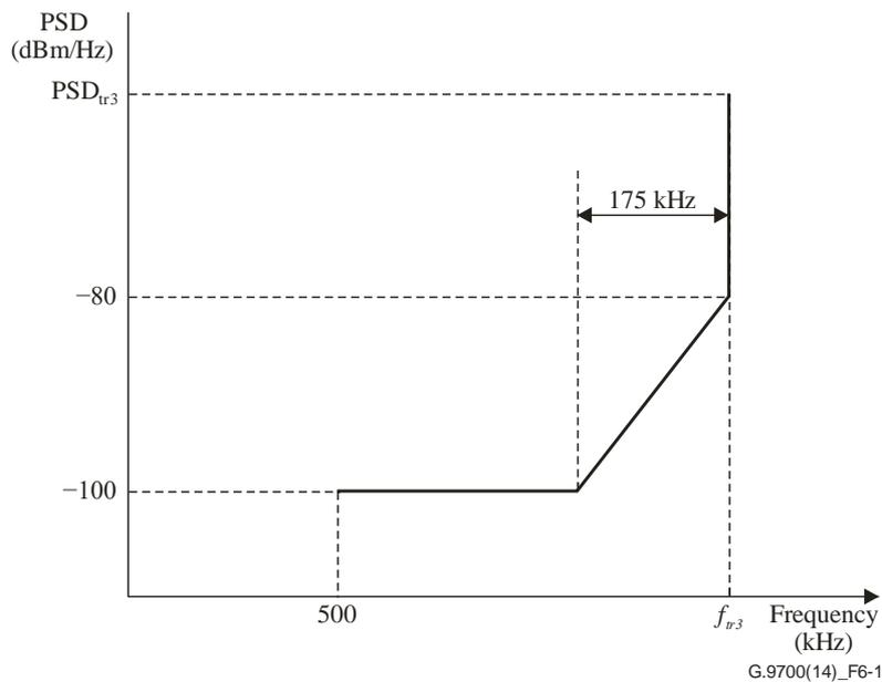
**Figure 6-1 – Low-frequency edge stop-band mask**
