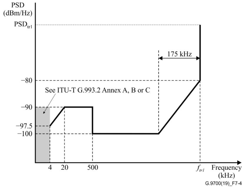
**Figure 7-4 – Low-frequency edge out-of-band LPM**
