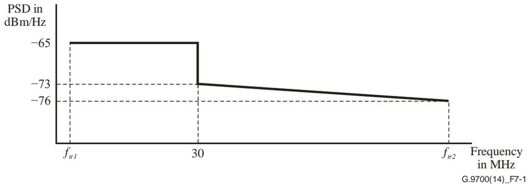
**Figure 7-1 – In-band limit PSD mask LPM\_106**
