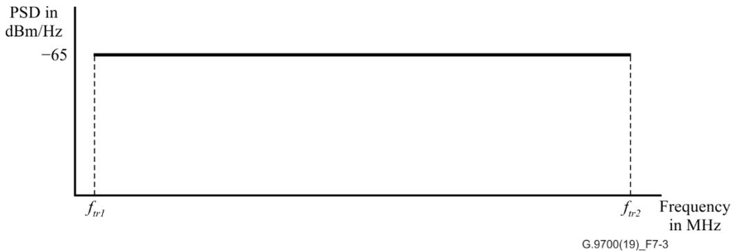
**Figure 7-3 – In-band limit PSD mask LPM\_106high**
