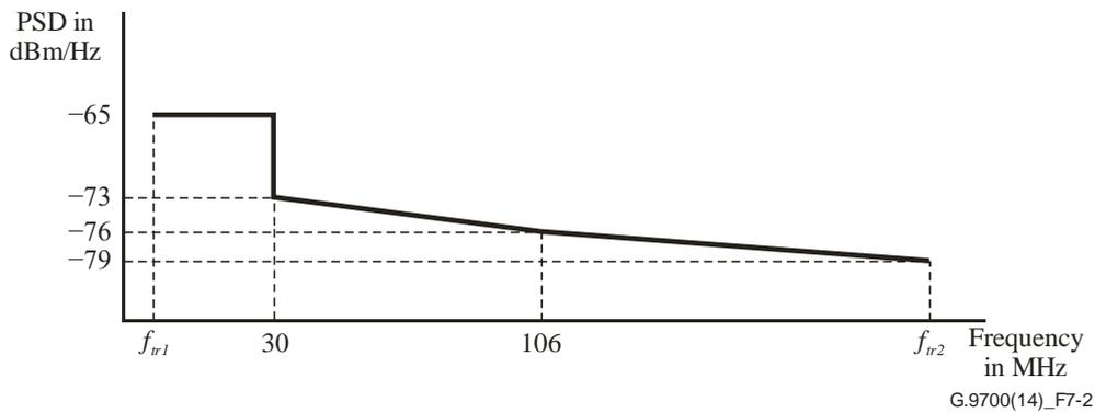
**Figure 7-2 – In-band limit PSD mask LPM\_212**
