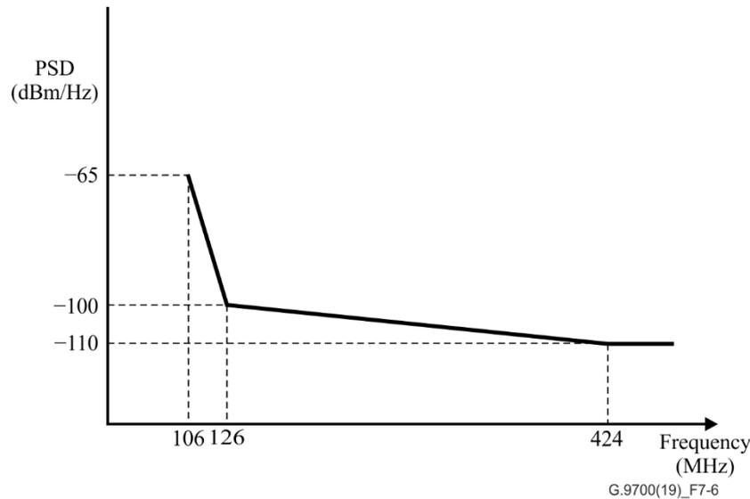
**Figure 7-6 – High-frequency edge out-of-band LPM to be used in combination with LPM\_106high**
