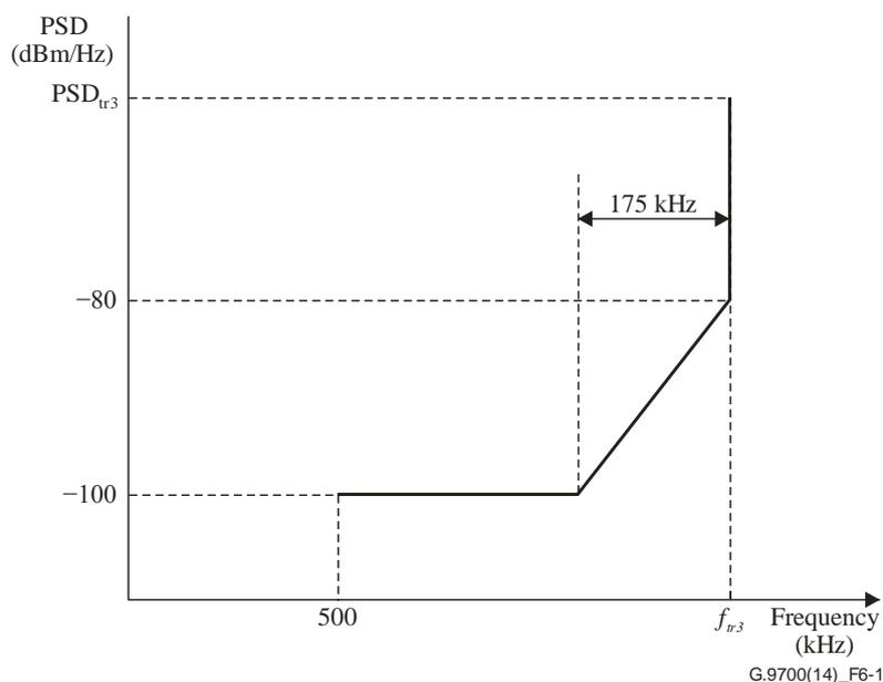
**Figure 6-1 – Low-frequency edge stop-band mask**
