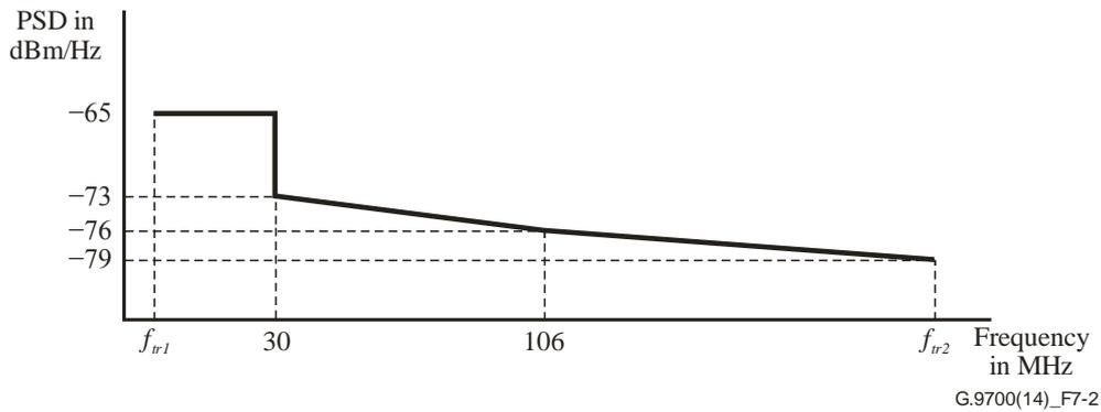
**Figure 7-2 – In-band limit PSD mask for 212 MHz profile**
