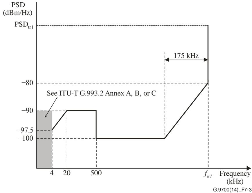
**Figure 7-3 – Low-frequency edge out-of-band LPM**
