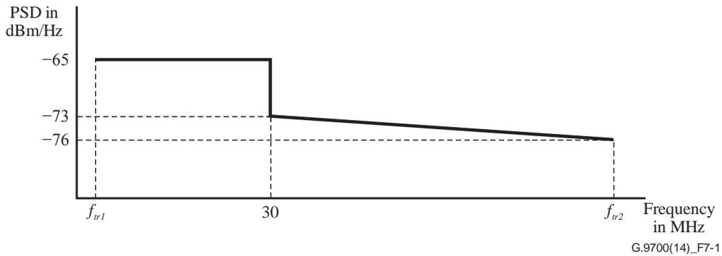
**Figure 7-1 – In-band limit PSD mask for 106 MHz profile**
