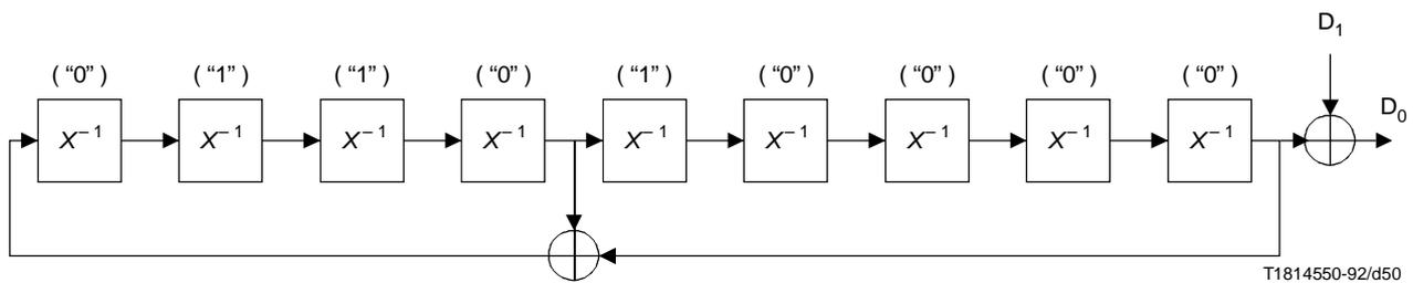
NOTE – At the beginning of a frame all register cells are cleared and loaded with initial values defined above each register as (“0”) or (“1”) in the figure.
