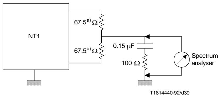
a) These resistors should be better than 0.1% tolerance.
