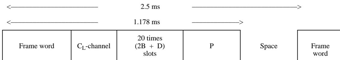
P Parity bit: The P bit is used to get an even number of "1"s in a frame; so it is set to "1" or "0" when the number of "1" s in a frame is odd or even, respectively.
