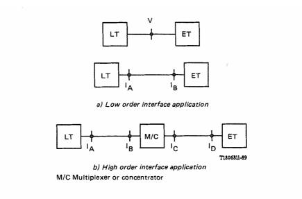
$\mathit{Note}-I_B$  and  $I_A$  are the interface points supporting  $V_1$  or  $V_3$  interfaces.  $I_C$  and  $I_D$  are the interface points supporting  $V_2$  or  $V_4$  interfaces.
