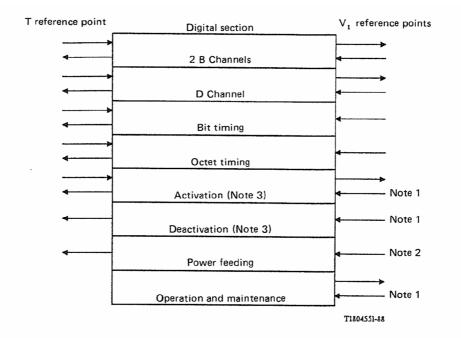
Note 1 – These functions are conveyed by the C<sub>V1</sub> channel across the V<sub>1</sub> reference point.
