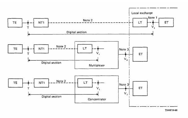
Note 1 — The LT may be integrated together with the ET or separate (as integral part or outside of the local exchange). Note 2 — In case of a digital section using a digital transmission system for metallic pairs the application of one regenerator may be foreseen. Note 3 — Local and remote applications are envisaged. For the remote case a transparent link between the remote multiplexer or concentrator and the local exchange will be used.
