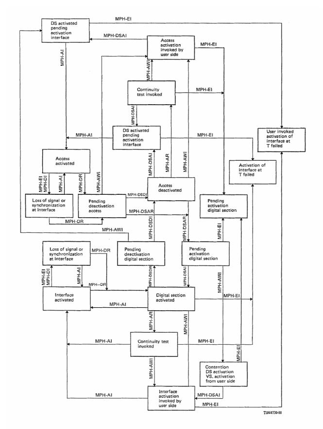
Note – The actions to be taken when entering the states "Loss of signal or synchronization at interface", "Activation of digital section failed", "Activation of interface at T failed" and "User invoked activation of interface at T failed" require further study.
