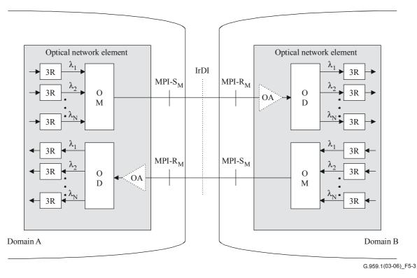
Figure 5-3/G.959.1 – Multichannel IrDI applications using preamplifiers
