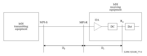
Figure 7-3/G.959.1 – Single channel IrDI with dispersion compensation (DC) in the receiver
