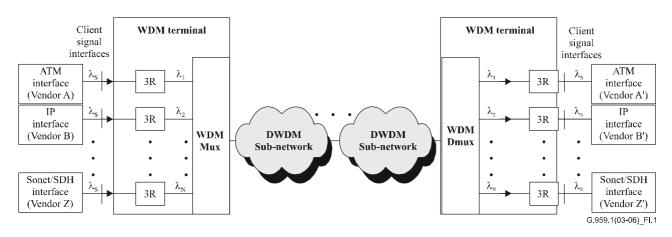
Figure I.1/G.959.1 – Example of client signal interface with 3R regeneration
