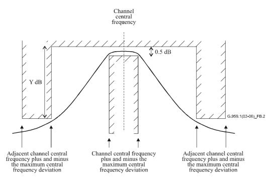
Figure B.2/G.959.1 – Optical bandpass filter frequency response
