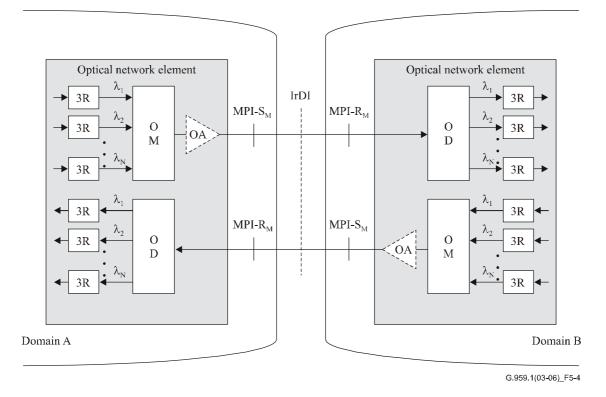
Figure 5-4/G.959.1 – Multichannel IrDI applications using booster amplifiers
