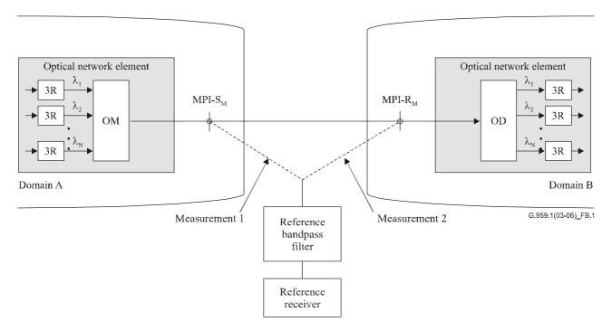
Figure B.1/G.959.1 – Method B configuration
