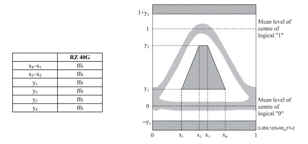
Figure 7-2/G.959.1 – Mask of the eye diagram for RZ 40G optical transmit signal
