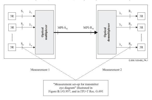
Figure A.1/G.959.1 – Method A configuration
