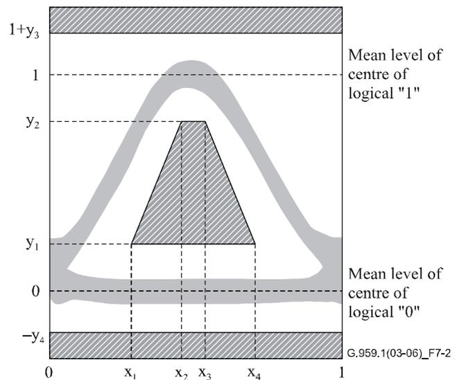
**Figure 7-2/G.959.1 – Mask of the eye diagram for RZ 40G optical transmit signal**
