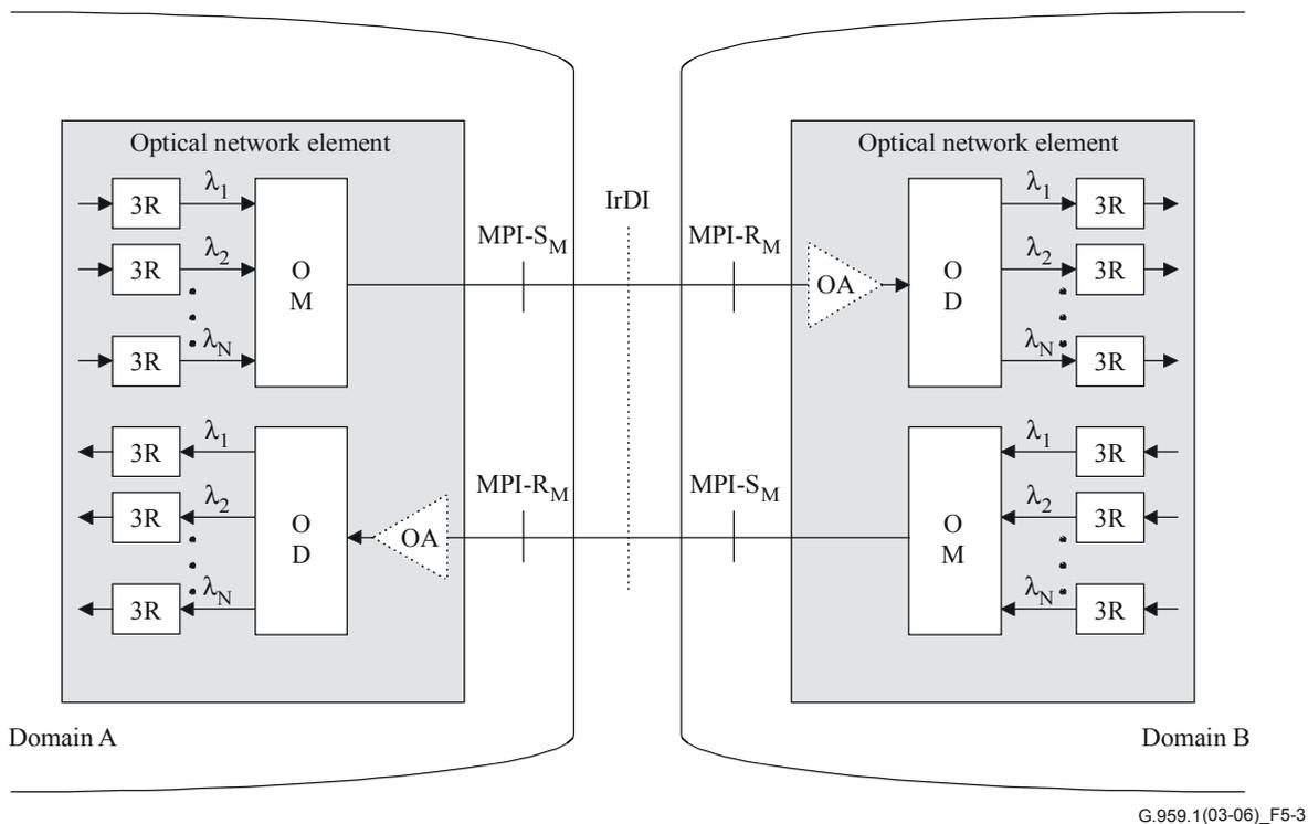
**Figure 5-3/G.959.1 – Multichannel IrDI applications using preamplifiers**
