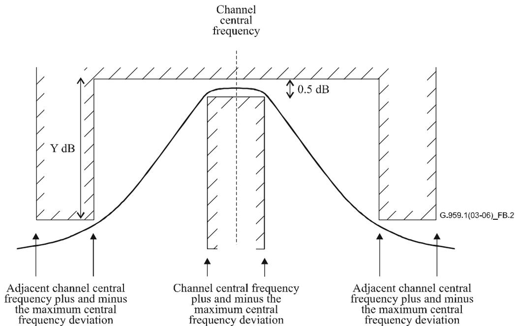
**Figure B.2/G.959.1 – Optical bandpass filter frequency response**
