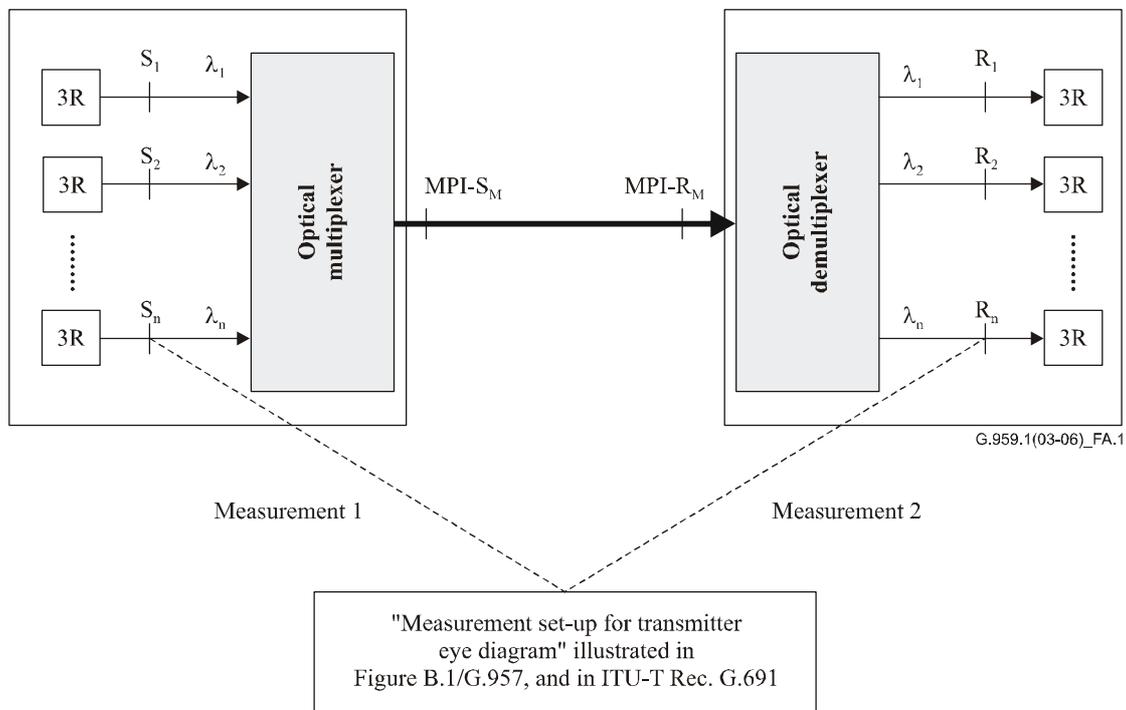
Figure A.1/G.959.1 – Method A configuration
