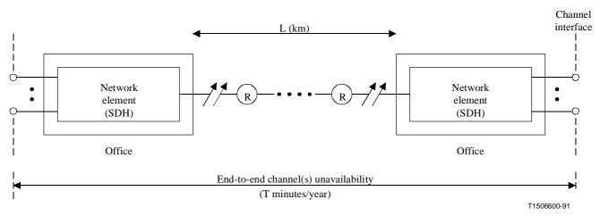
b) Reference circuit for end-to-end channel(s) unavailability in SDH systems
