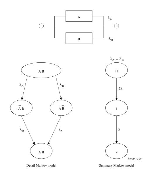
Figure 2/G.911 – Examples of reliability block diagrams
