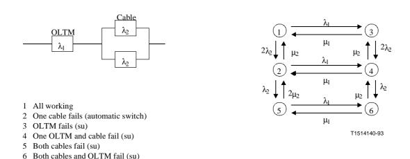
Figure III.5/G.911 – Connection with cable redundancy and its Markov model
