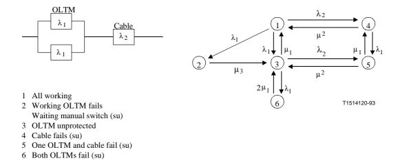
Figure III.3/G.911 – Connection with terminal equipment redundancy and manual switchover and its Markov model
