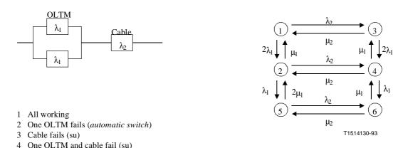
Figure III.4/G.911 – Connection with terminal equipment redundancy and automatic switchover and its Markov model
