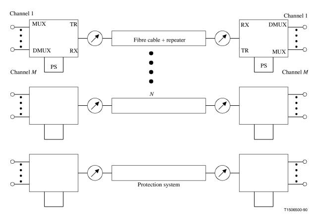
Figure II.1/G.911 – Example – System configuration "N + 1" ("N" active and 1 reserve)
