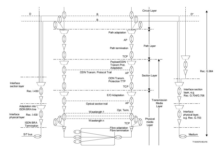
FIGURE II.1/G.902 An example of a functional model of an Optical Access Network based on Recommendation G.964
