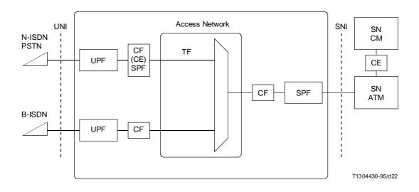
FIGURE III.3/G.902 Remotely connected access
