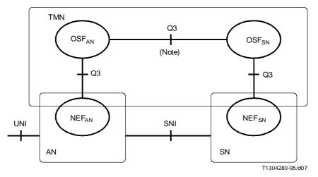
$\ensuremath{\text{NOTE}}$  – In case of different operators this Q3 reference point becomes an x reference point.
