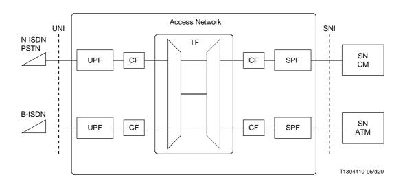
FIGURE III.1/G.902 Multiplexing on transmission physical media layer
