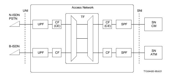
FIGURE III.2/G.902 Remote access connection
