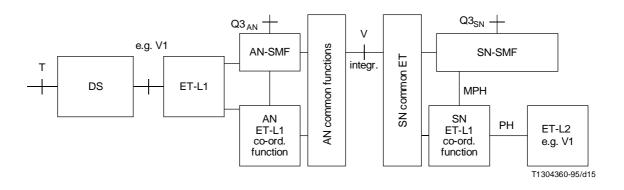
FIGURE A.5/G.902 The common ET and the individual ET
