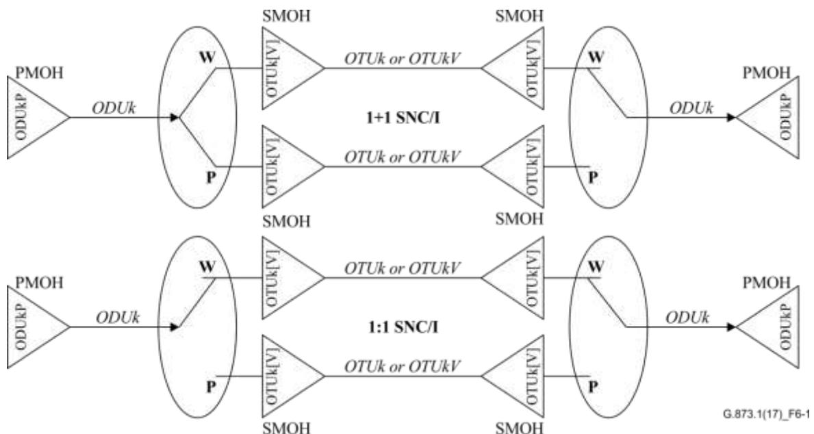
Figure 6-1 – OTUk or OTUkV monitored ODUk SNC/I protection configuration
