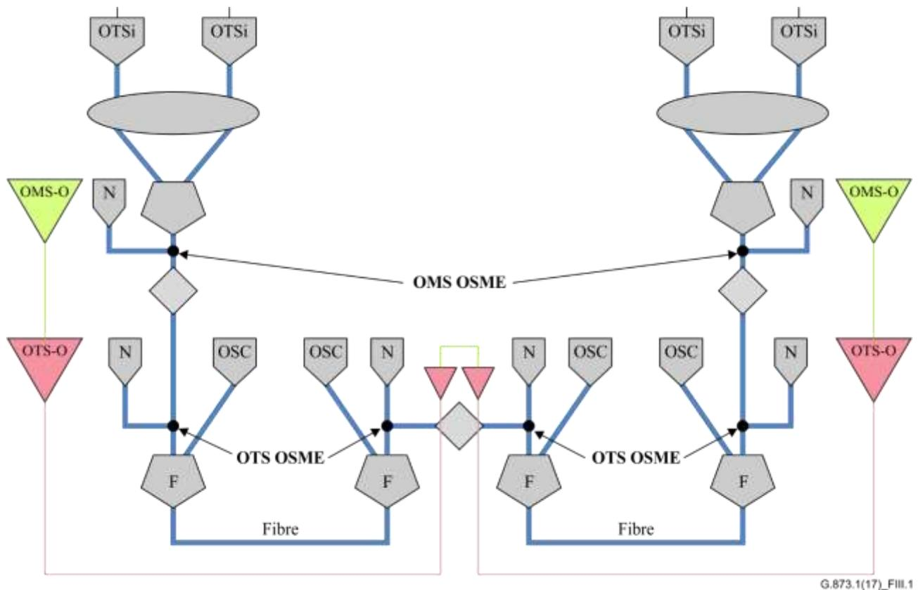
Figure III.1 – Network with OTS and OMS optical signal maintenance entities (OSME)
