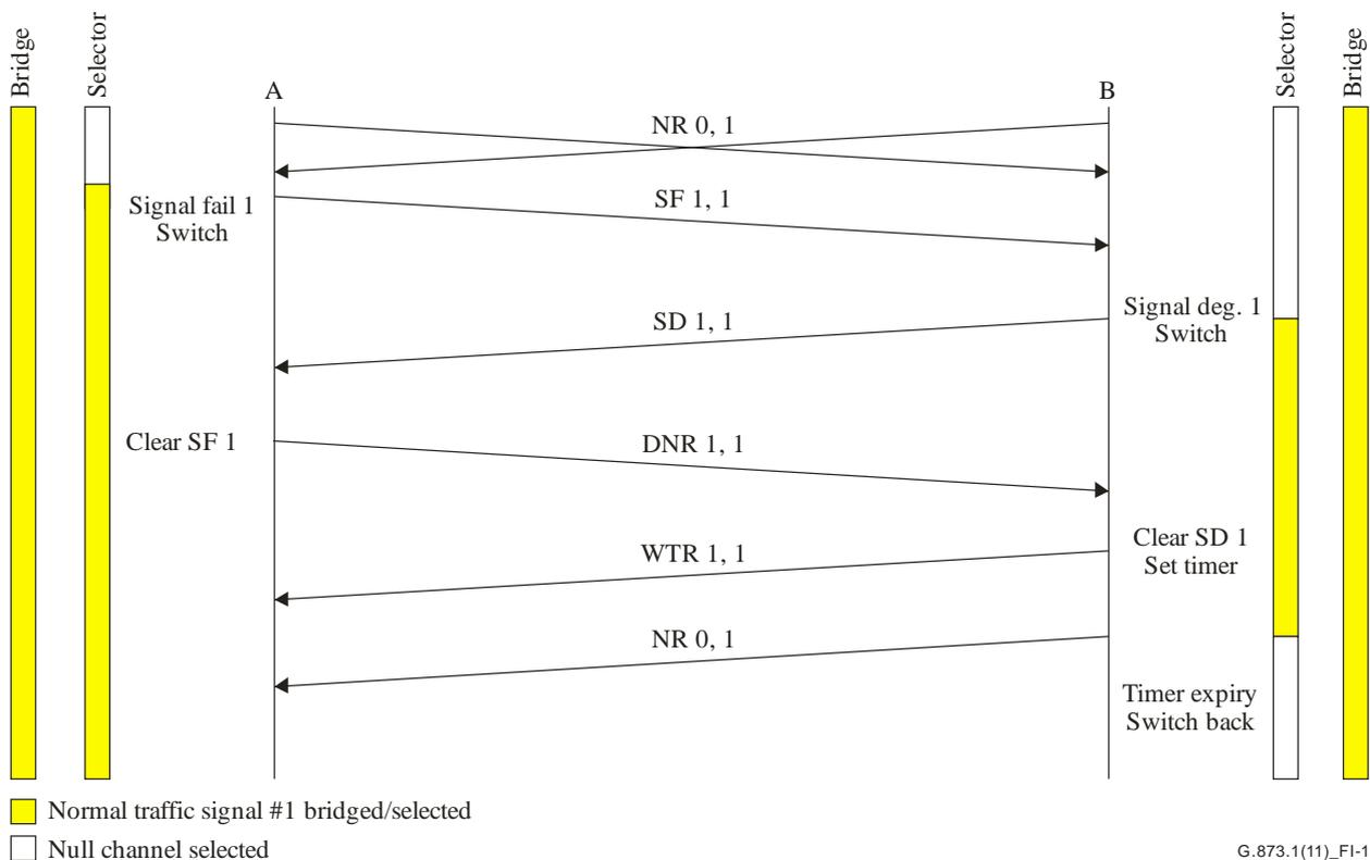
Figure I.1 – Example APS message flow for 1+1 unidirectional switching
