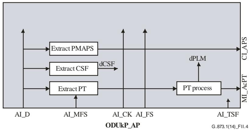
**Figure II.4 – Supporting ODUk PM APS access in ODUk/GBR adaptation sink functions**
