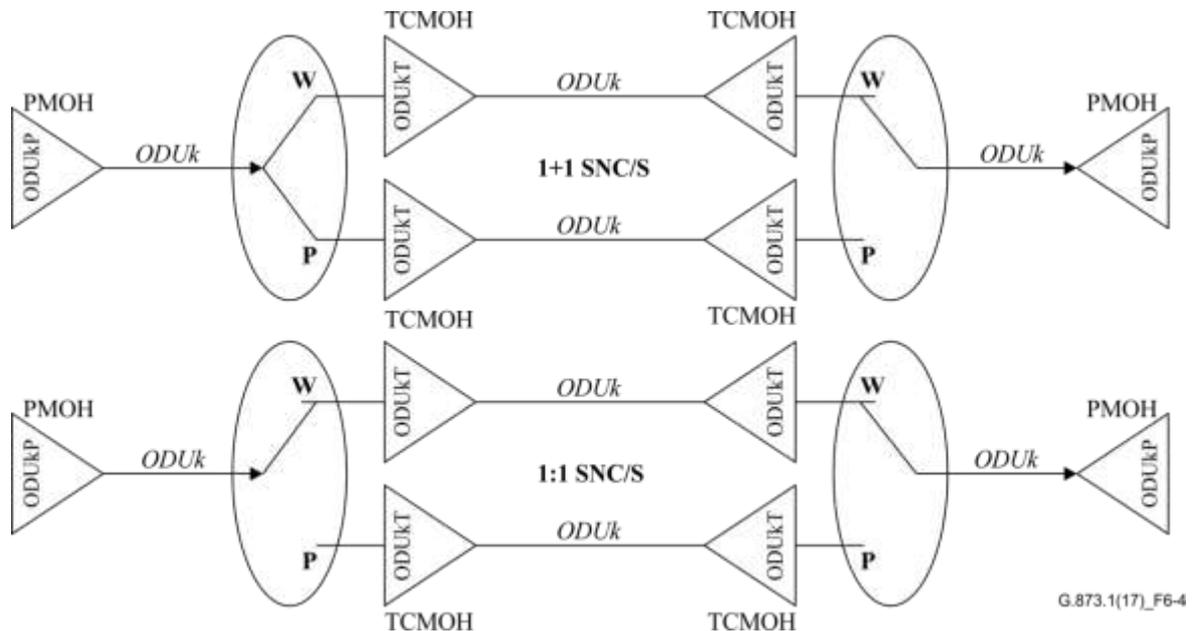
**Figure 6-4 – ODUkT monitored SNC/S protection configuration**
