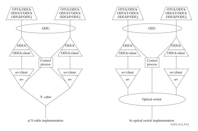
Figure II.2 – OTN client SNC/I protection models
