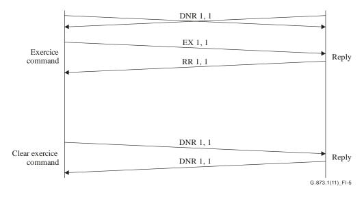
Figure I.5 – Example of Exercise command from 1+1 DNR state
