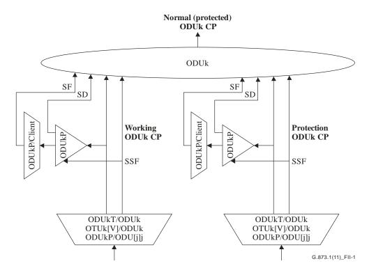
Figure II.1 – SNC/Nc protection atomic functions
