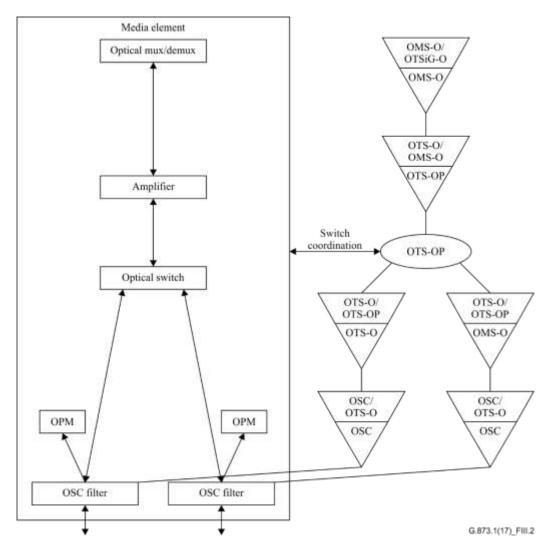
Figure III.2 – OTS OSME protection
