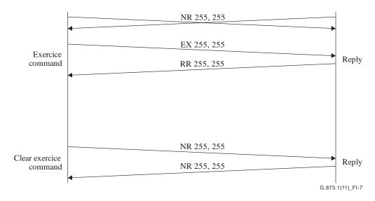
Figure I.7 – Example of Exercise command from 1:n NR state with extra traffic
