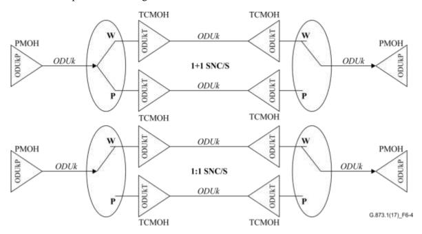
Figure 6-4 – ODUkT monitored SNC/S protection configuration
