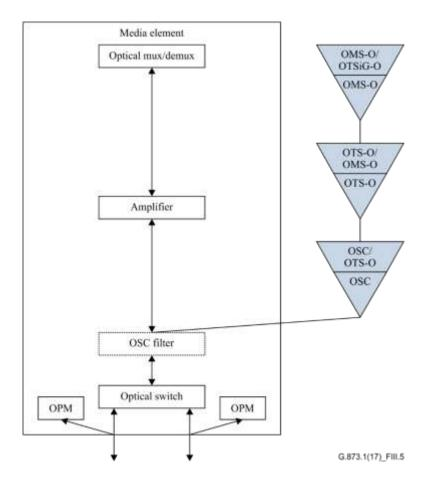
Figure III.5 – Media protection below the OSC filter
