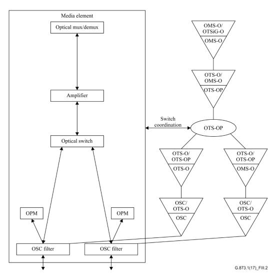
Figure III.2 – OTS OSME protection
