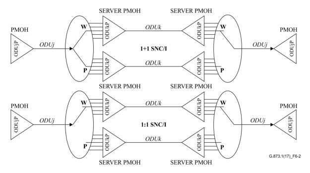
Figure 6-2 – Server ODUk monitored ODU[i]j/ODUj SNC/I protection configuration
