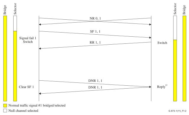
a) Historically, DNR was acknowledged with RR. Here, answering DNR with DNR makes no fundamental difference in the states of the two sides and it allows for a meaningful exercise implementation.
