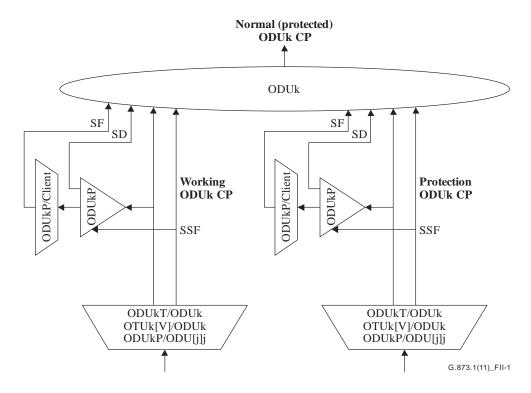
Figure II.1 – SNC/Nc protection atomic functions
