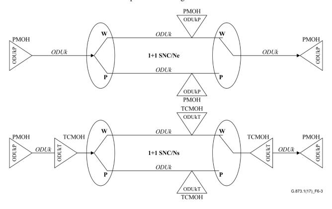
Figure 6-3 – ODUkP non-intrusively monitored ODUk SNC/Ne and ODUkT monitored ODUk SNC/Ns protection configurations
