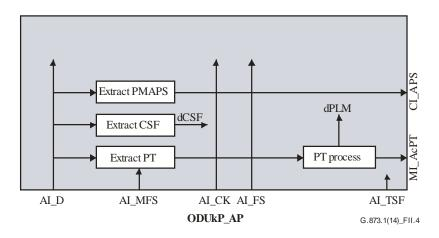
Figure II.4 – Supporting ODUk PM APS access in ODUkP/CBR adaptation sink functions
