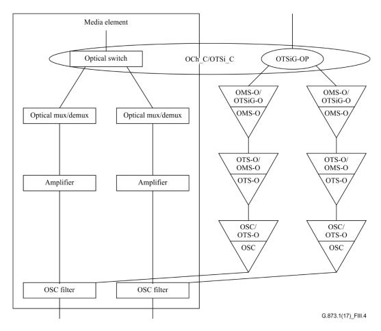
Figure III.4 – OCh or OTSi SNC protection
