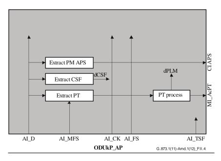
Figure II.4 – Supporting ODUk PM APS access in ODUkP/CBR adaptation sink functions
