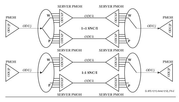
Figure 5-2 – Server ODUk-monitored ODU[i]j/ODUj SNC/I protection configuration
