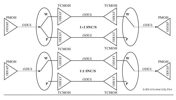
Figure 5-4 – ODUkT-monitored SNC/S protection configuration
