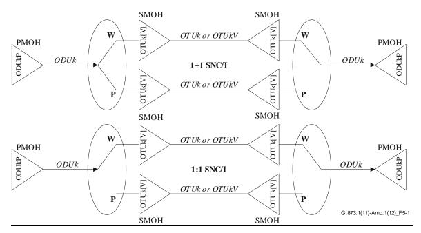
Figure 5-1 – OTUk- or OTUkV-monitored ODUk SNC/I protection configuration
