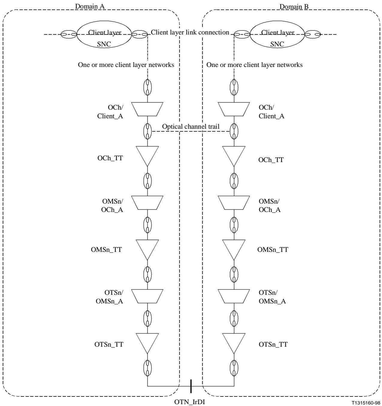
**Figure 10/G.872 – Scenario 2: Interconnection of different administrative domains via an optical island with an OTN inter-domain interface**
