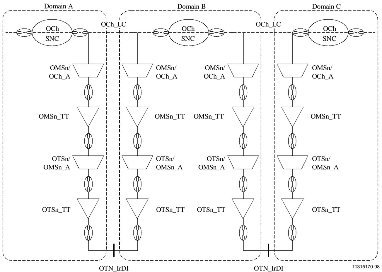
**Figure 11/G.872 – Scenario 3: Interconnection of OTN subnetworks in different administrative domains via an OTN inter-domain interface supporting OCh interworking**
