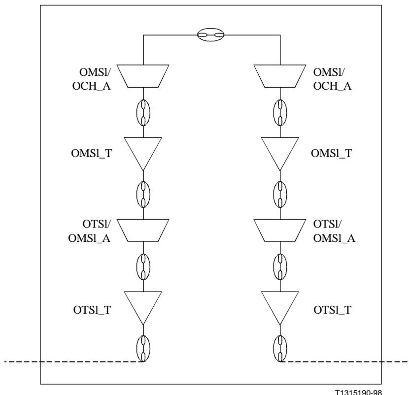
Figure I.1/G.872 – Example of optical wavelength conversion
