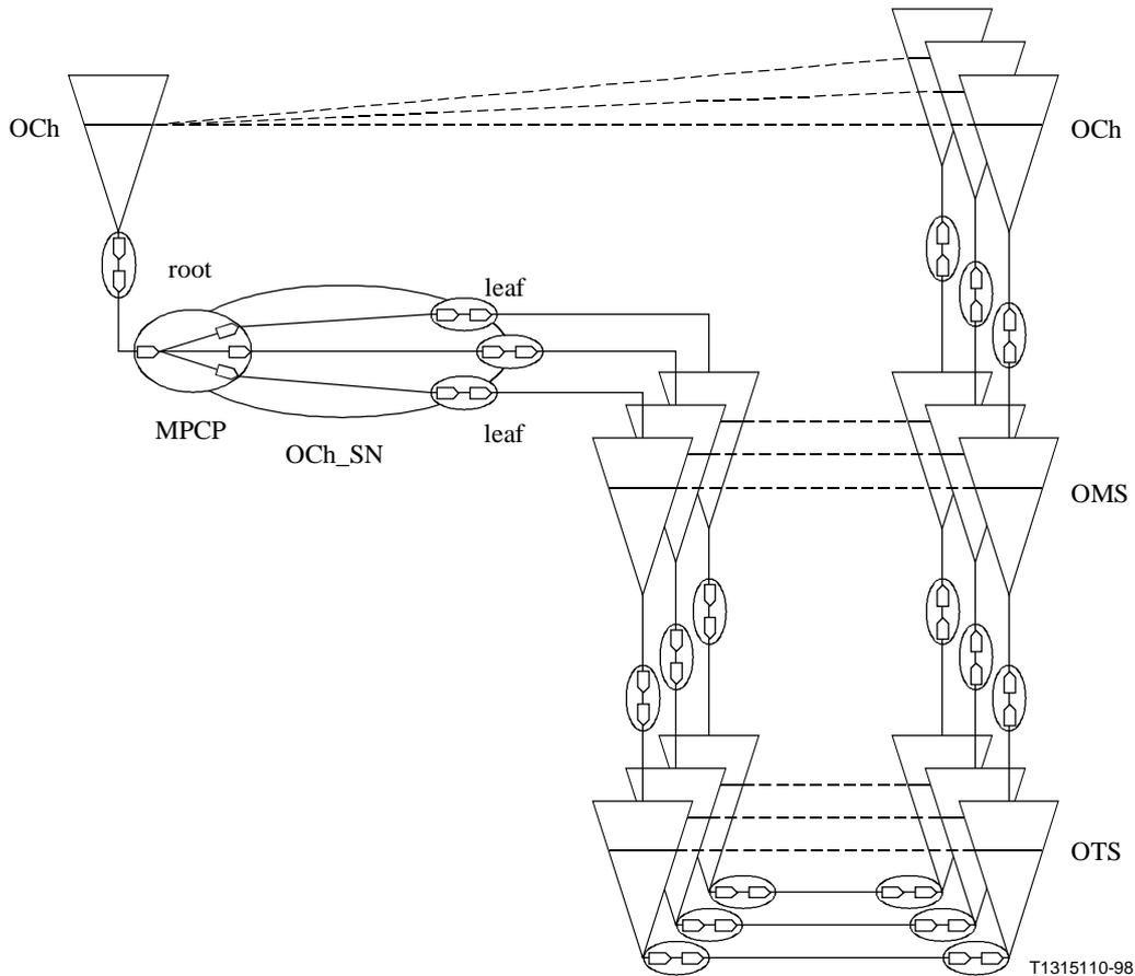
**Figure 5/G.872 – Point-to-multipoint optical channel connection**
