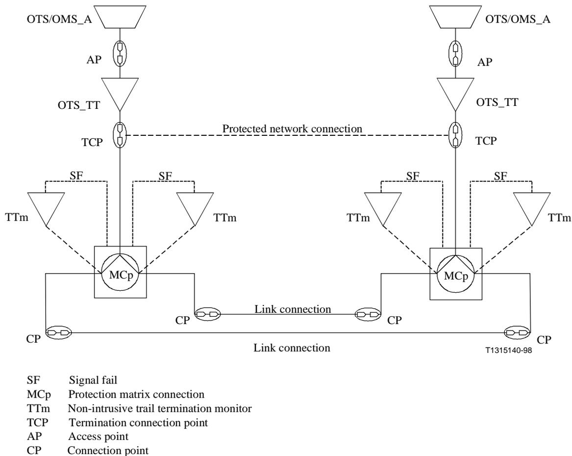
**Figure 8/G.872 – Network connection protection with non-intrusive monitoring in the optical transmission section layer network**
