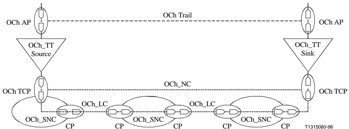
**Figure 2/G.872 – OCh layer network example**
