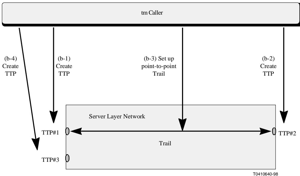
**Figure B.2/G.852.2 – Creation of a trail and TTPs of a server layer network**
