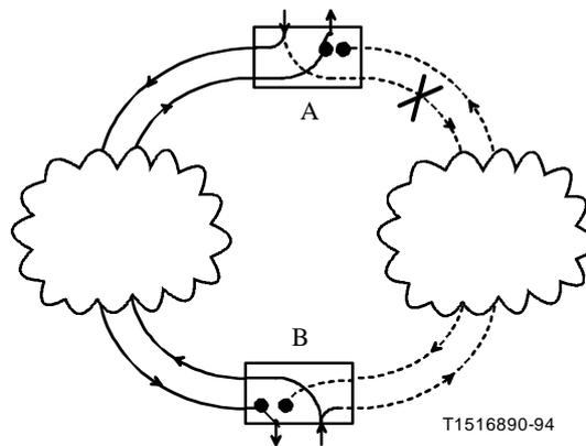
c) Unidirectional failure – Fibre 2
