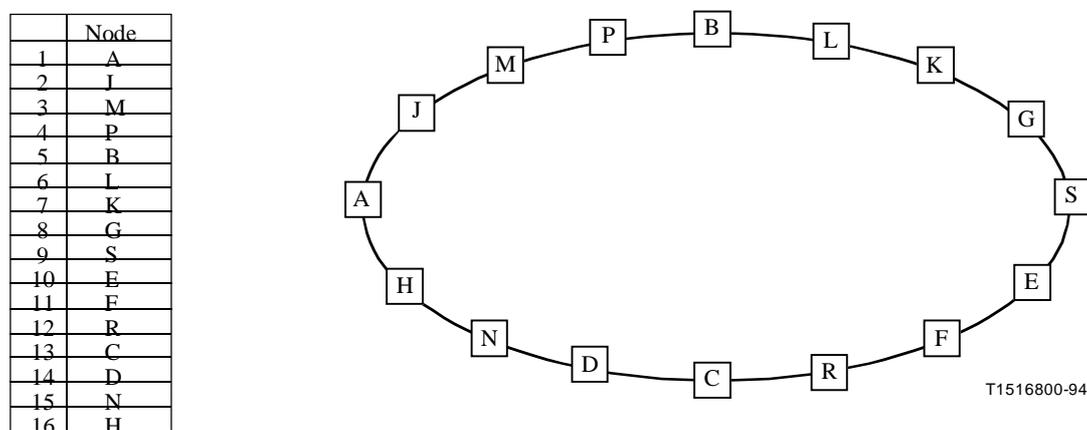
Figure 7-5/G.841 – Conceptual representation of a ring topology map
