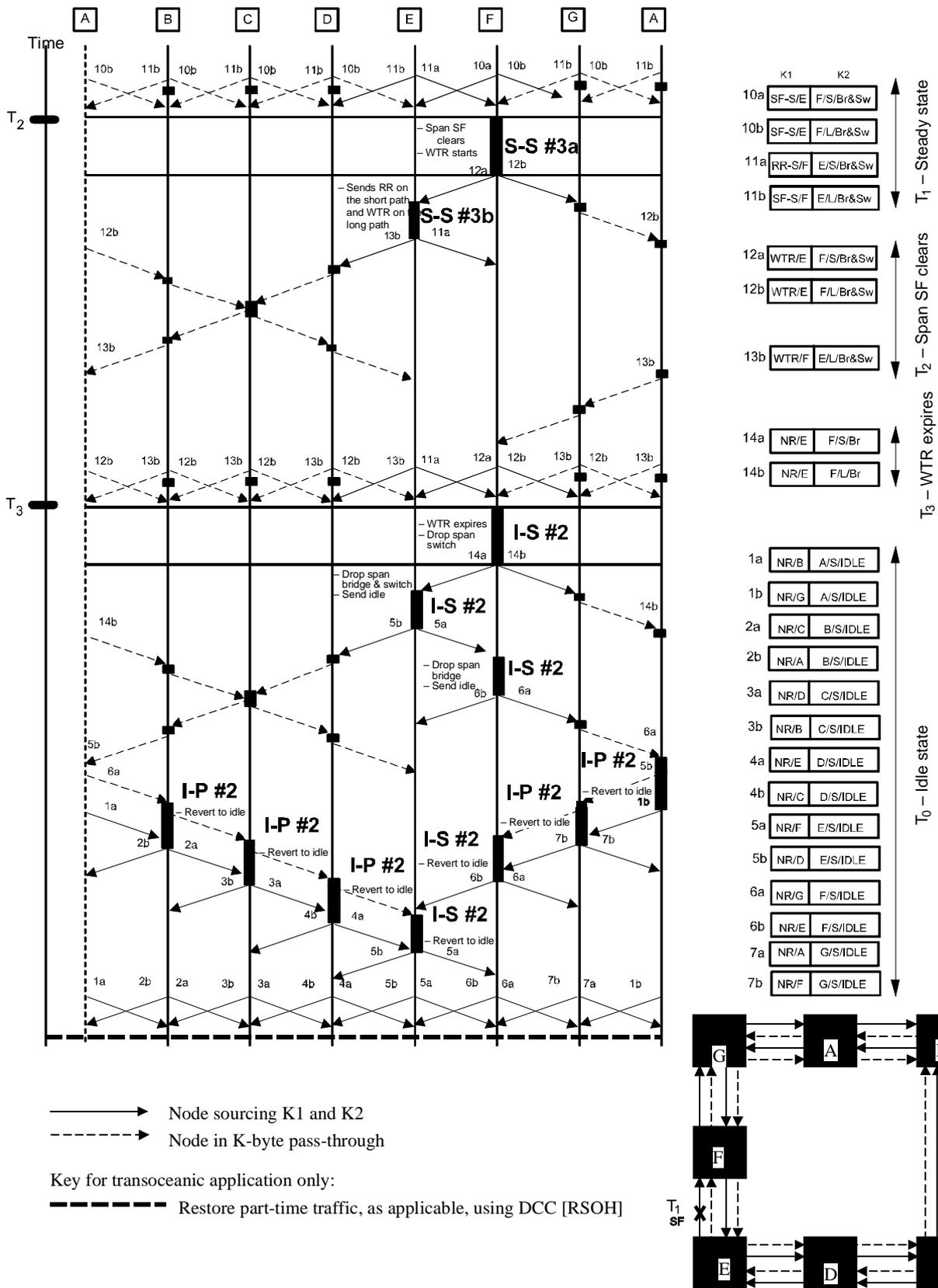
Figure I.1/G.841 – Four-fibre MS shared protection ring – Unidirectional failure (span) on working from E to F (concluded)
