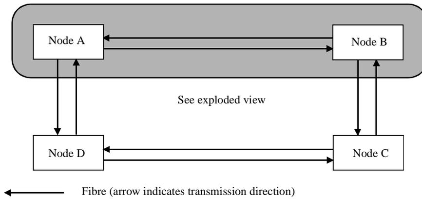
NOTE – Each fibre carries both working and protection traffic, as shown in the exploded view.
