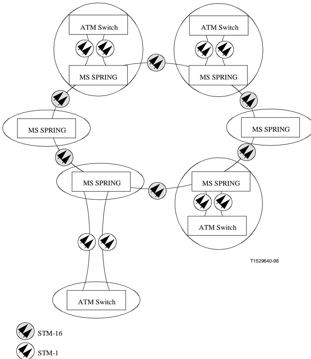
**Figure 6-4/G.841 – NUT Channels supporting HO VC connectivity among ATM switches**
