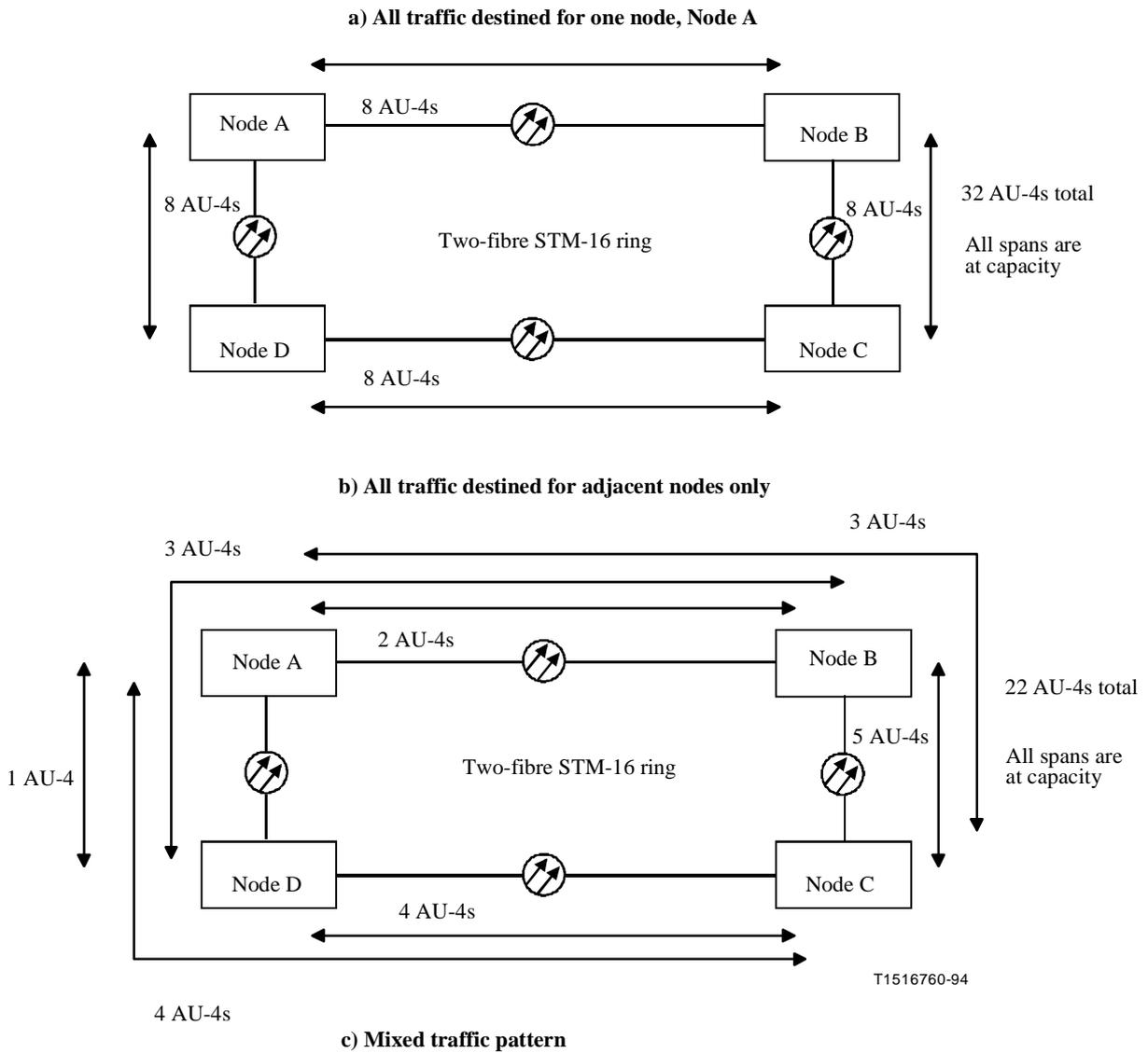
Figure 6-1/G.841 – Effects of demand pattern on capacity of bidirectional MS shared protection rings
