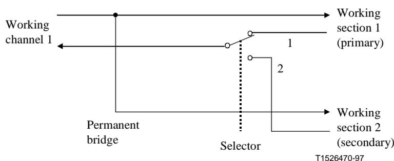
**Figure B.1/G.841 – MSP Switch – 1 + 1 bidirectional switching, optimized (shown in released position with working section 1 as primary)**
