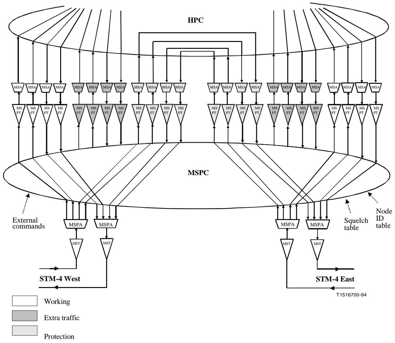
**Figure 5-3/G.841 – Functional model for a two-fibre MS shared protection ring – Pass-through state**
