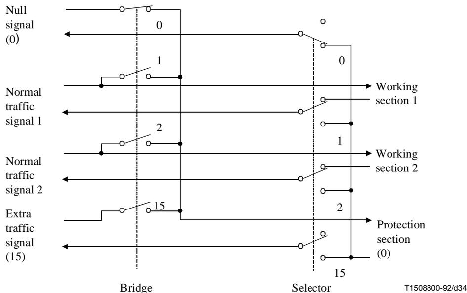
**Figure 7-1/G.841 – MSP switch – 1:n architecture (shown in released position)**
