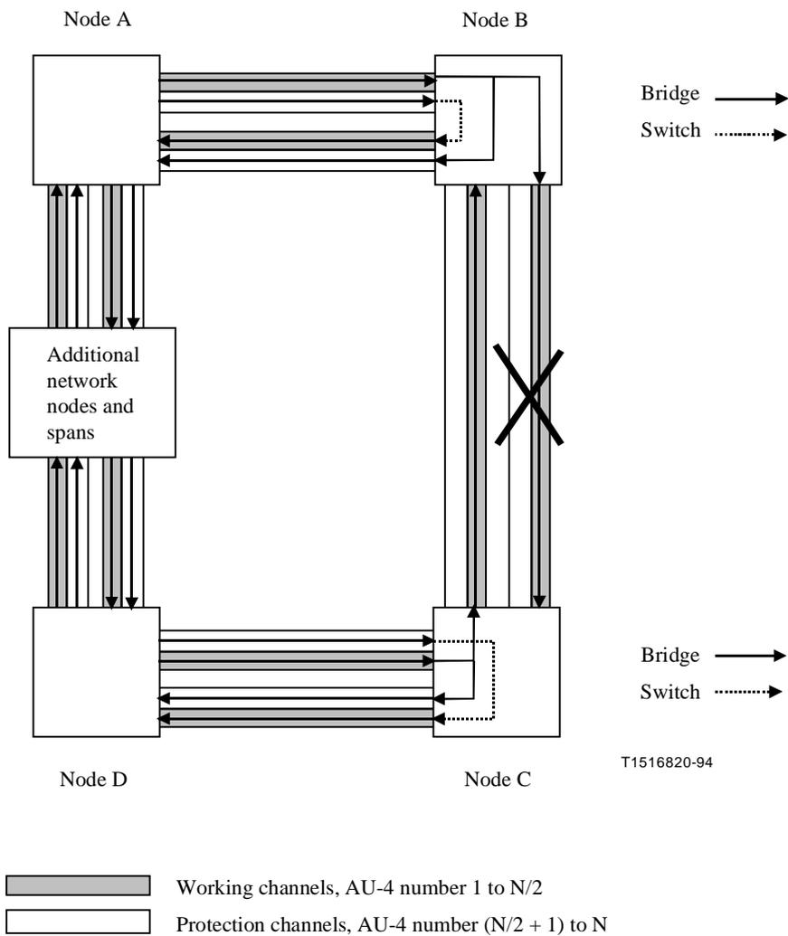
**Figure 7-7/G.841 – Bridge and switch in a two-fibre MS shared protection ring**
