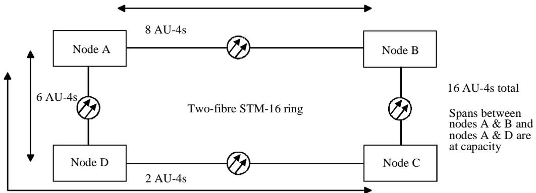
NOTE – Since all the traffic is destined for node A, and the span between node A and node B is full, traffic from node C routes through node D, leaving the span between node B and node C vacant.
