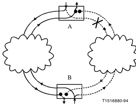
c) Unidirectional failure – Fibre 2
