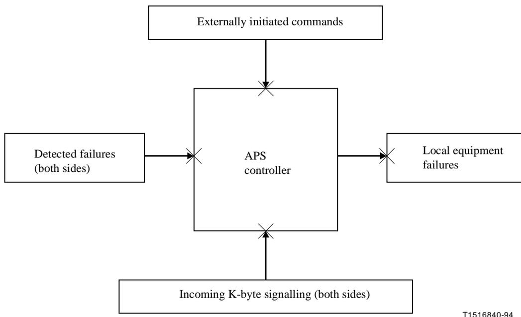
**Figure 7-9/G.841 – Conceptual MS shared protection ring APS controller**
