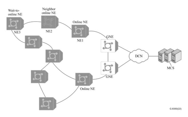
Figure B.1 – An example of an MTN network including a DCN
