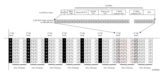
Figure A.5 – LLDP organizationally specific TLVs transmission channel over MTNS MCC
