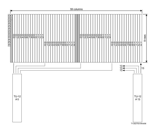
FIGURE 3-1/G.832 Support of 14 TU-12 s in 34 368 kbit/s
