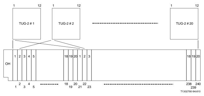
FIGURE 3-5/G.832 Multiplexing of 20 × TUG/2 into the 139 264 kbit/s payload capacity
