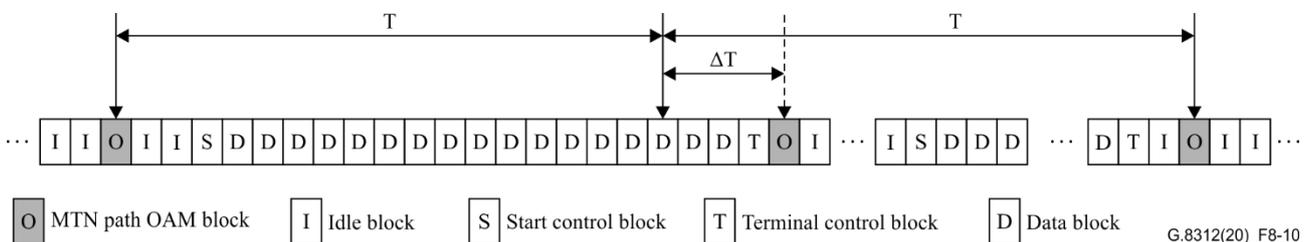
**Figure 8-10 – MTNP OAM block insertion illustration**
