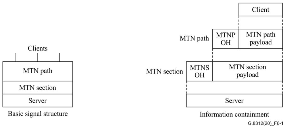
**Figure 6-1 – Basic signal structure and information containment relationships for an MTN**
