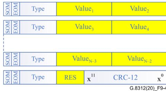
Figure 9-4 – Message bytes covered by a CRC
