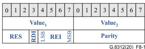
**Figure 8-1 – Value bytes in a basic message**
