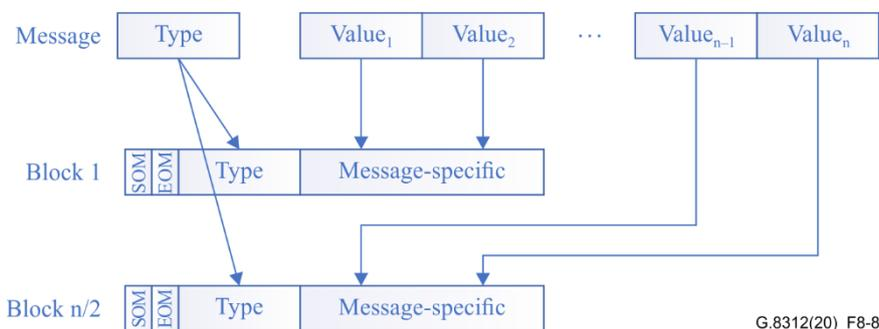
**Figure 8-8 – Mapping an MTNP OAM message into multiple MTNP OAM 66B blocks**
