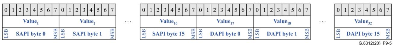
Figure 9-5 – TTI field of a CV message
