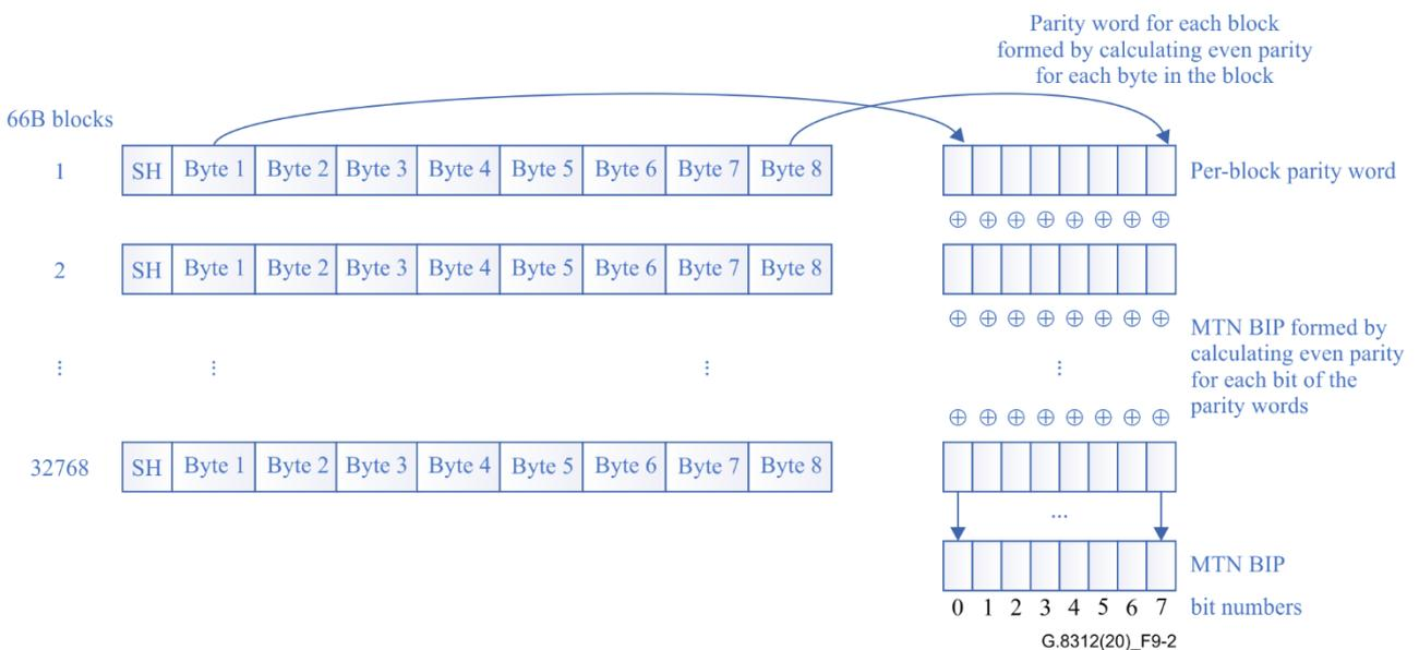
**Figure 9-2 – Parity calculation across a nominal 32K block interval**
