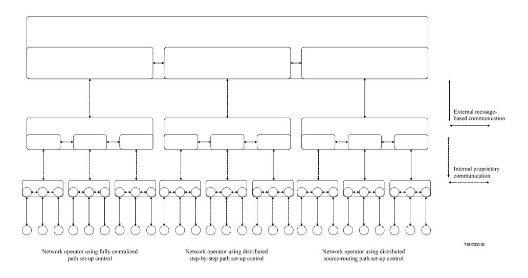
Figure 2/G.831 – Examples of specific path set-up control structures
