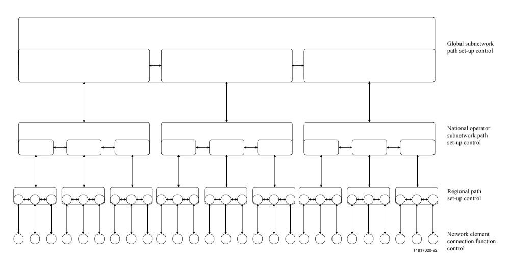
Figure 1/G.831 – Control structure for path set-up
