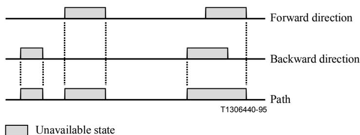
**Figure A.2/G.828 – Example of the unavailable state of a path**
