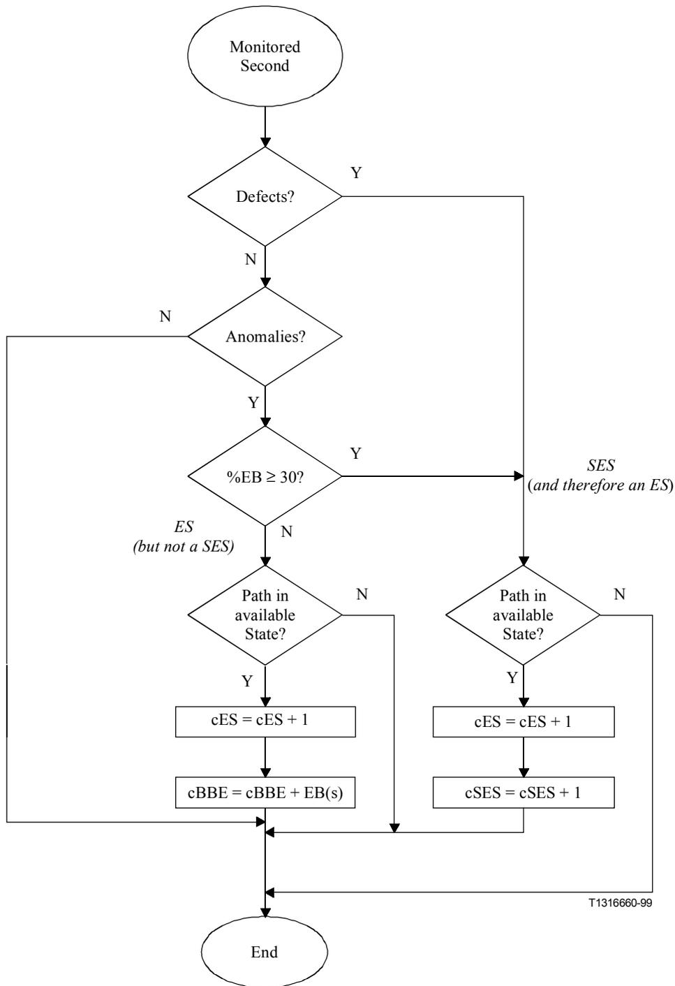
**Figure I.1/G.828 – Recognition of anomalies, defects, errored blocks, ES, SES and BBE**
