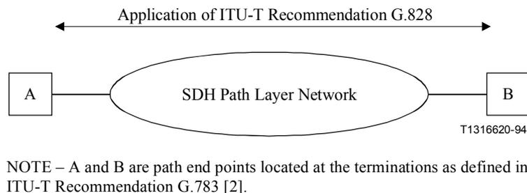
**Figure 1/G.828 – Application of ITU-T Recommendation G.828 for an end-to-end SDH path**
