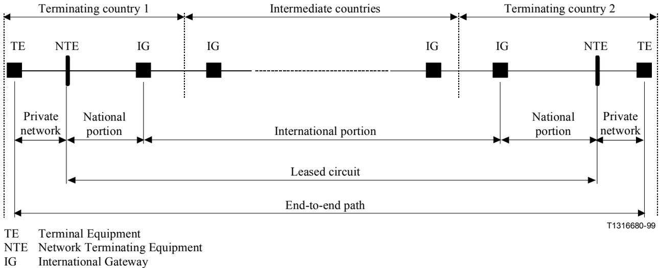
**Figure II.1/G.828 – Digital path composed of two private networks and a leased circuit provided by a public network operator**
