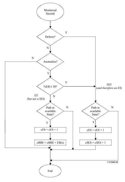
Figure I.1/G.828 – Recognition of anomalies, defects, errored blocks, ES, SES and BBE
