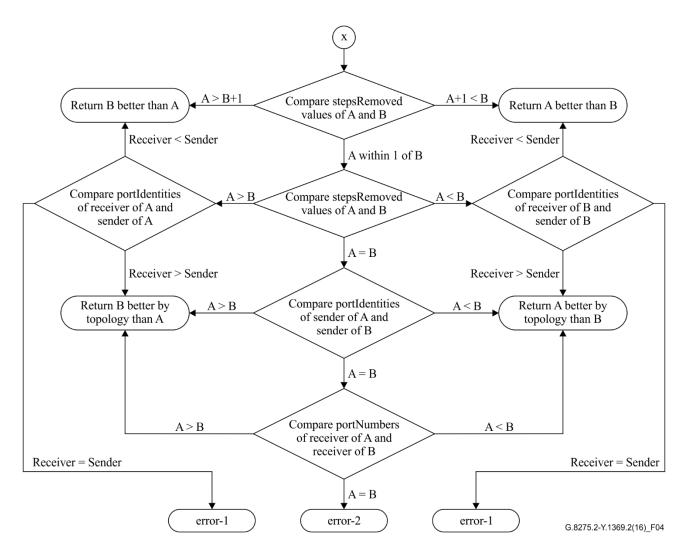
Figure 4 – Data set comparison algorithm, part 2, for Alternate BMCA
