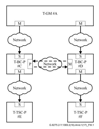
Figure III.1 – Steady-state, before A-D PTP connection failure
