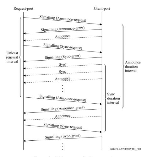
Figure 1 – Unicast negotiation example
