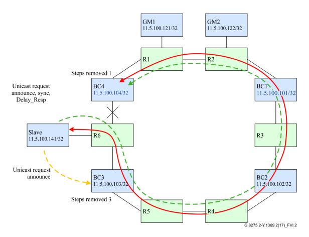
Figure VI.2 – Operation during a link failure between BC4 and R6
