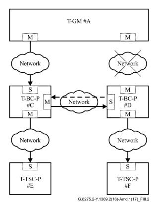
Figure III.2 – Steady-state, after A-D PTP connection failure
