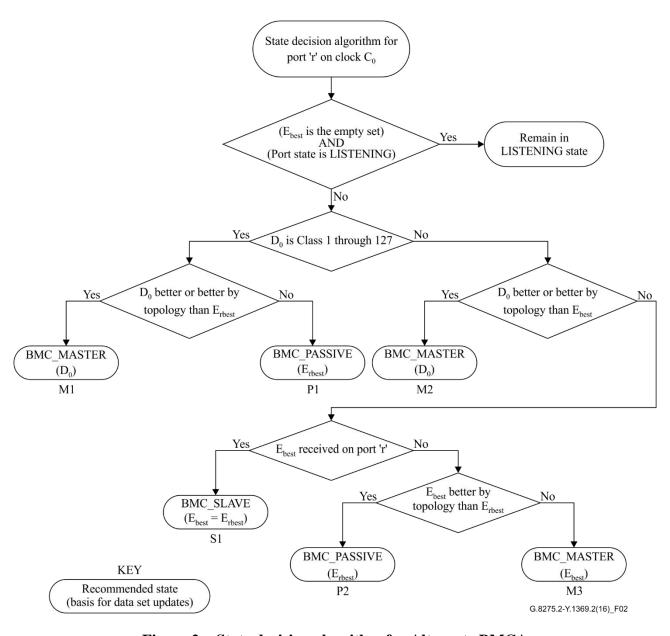
Figure 2 – State decision algorithm for Alternate BMCA
