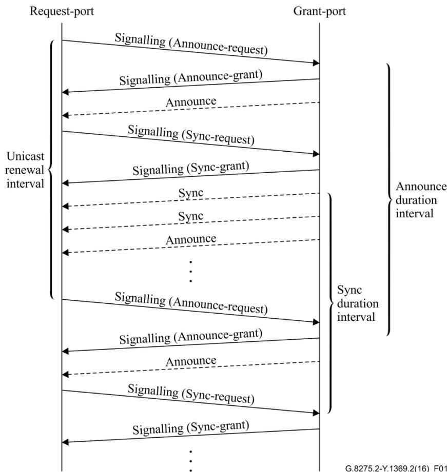
**Figure 1 – Unicast negotiation example**
