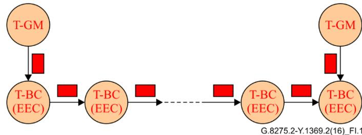
**Figure I.1 – Use of priority2 with two T-GMs in the network**
