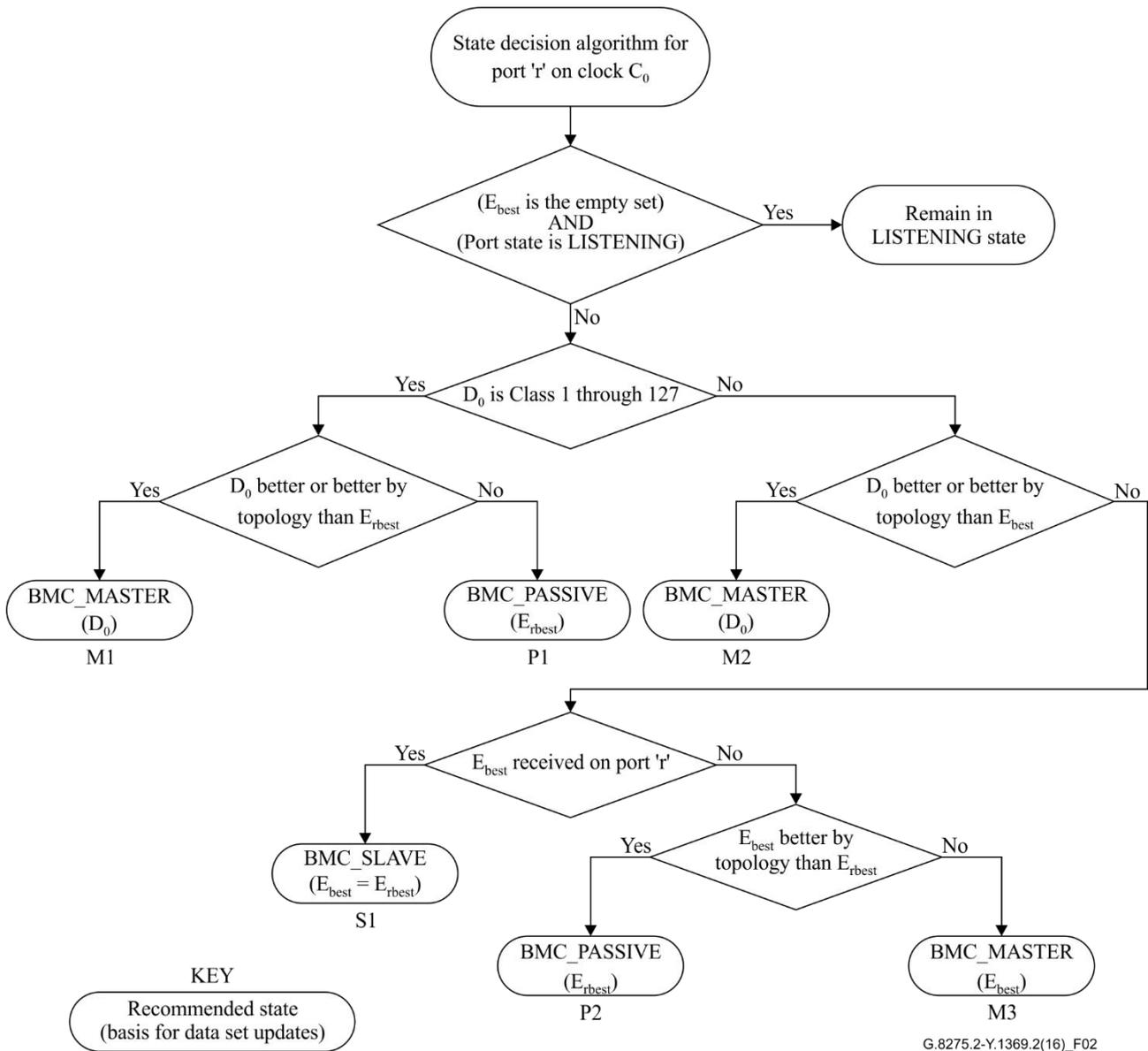
**Figure 2 – State decision algorithm for Alternate BMCA**
