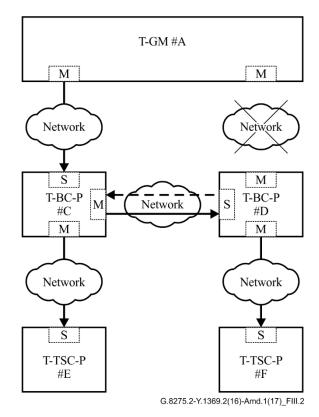
Figure III.2 - Steady-state, after A-D PTP connection failure
