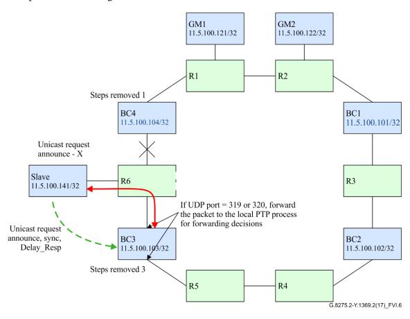
Figure VI.6 – Operation during the link failure if all PTP messages are terminated
