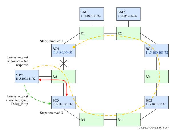
Figure VI.3 – Operation during a link failure between BC4 and R6 when static routes are used
