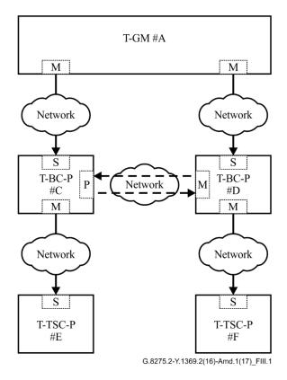
Figure III.1 – Steady-state, before A-D PTP connection failure
