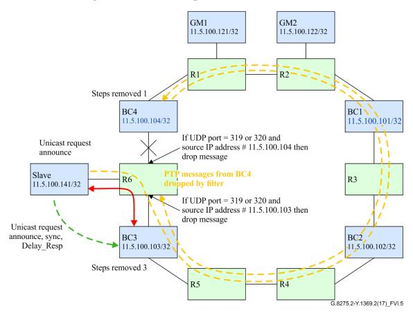
Figure VI.5 - Operation during a link failure between BC4 and R6 with IP filters in R6
