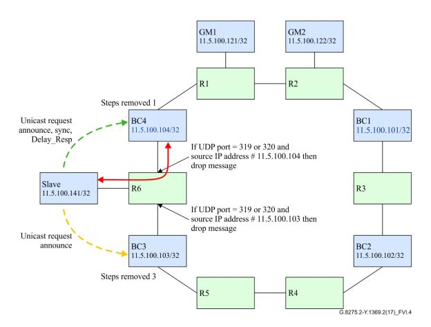
Figure VI.4 – Normal operation with IP filters in R6
