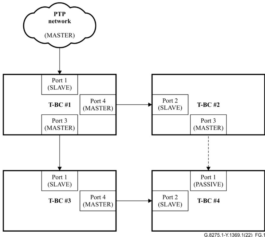
Figure G.1 – PASSIVE port monitors MASTER port
