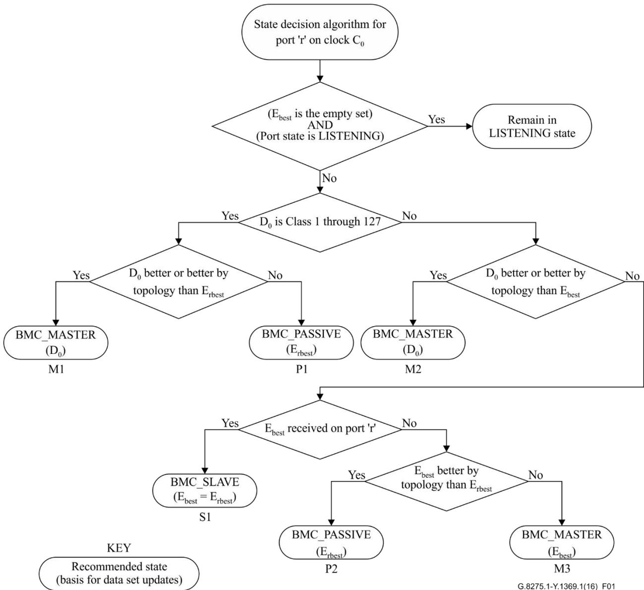
**Figure 1 – State decision algorithm for Alternate BMCA**
