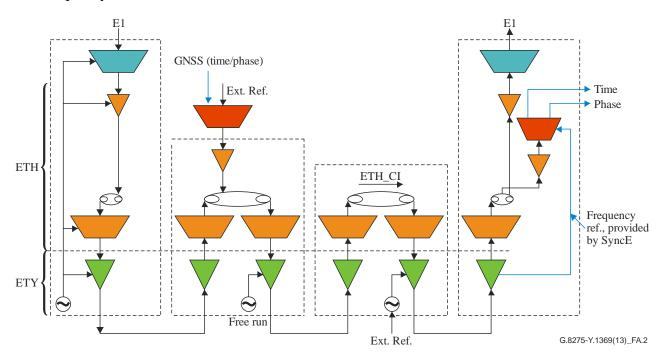
Figure A.2 – Time/phase with frequency support provided by the network (e.g., synchronous Ethernet)
