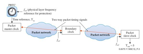
Figure I.3 – Protection using physical layer frequency references
