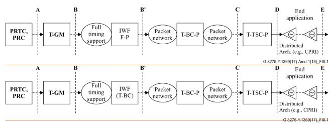
Figure III.1 – Deployment case requiring IWF
