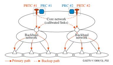
NOTE - T-GM are connected to the PRTC in this architecture
