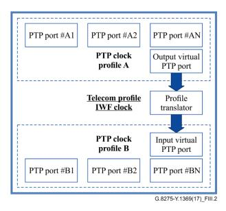
Figure III.2 – Model of telecom profile IWF clock
