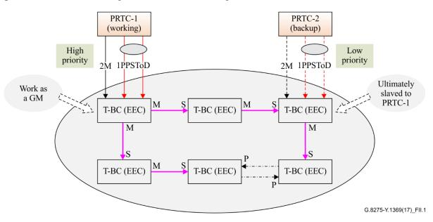
Figure II.1 – Normal state (T-BC connected to working PRTC is working as a GM)
