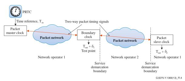
Figure I.4 – Timing transmission over a second operator's network
