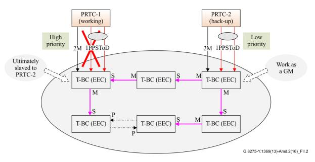
Figure II.2 – Abnormal state (the working PRTC has failed)
