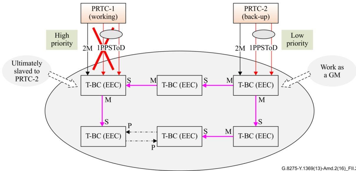
**Figure II.2 – Abnormal state (the working PRTC has failed)**
