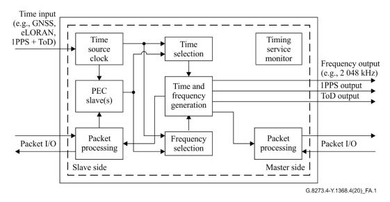
Figure A.1 – The T-TSC-A and T-BC-A functional model
