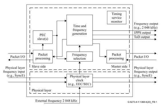
Figure B.1 – T-TSC-P and T-BC-P functional model
