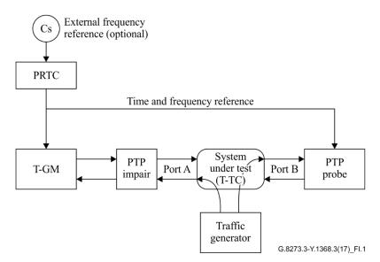
Figure I.1 – T-TC test set-up with cross traffic
