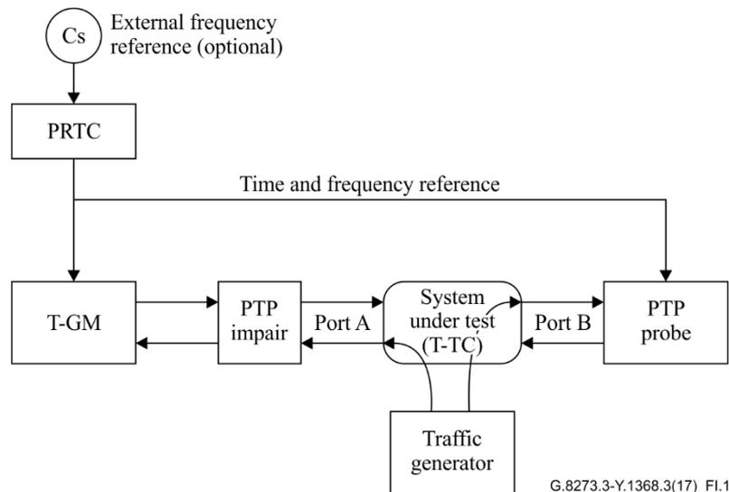
Figure I.1 – T-TC test set-up with cross traffic
