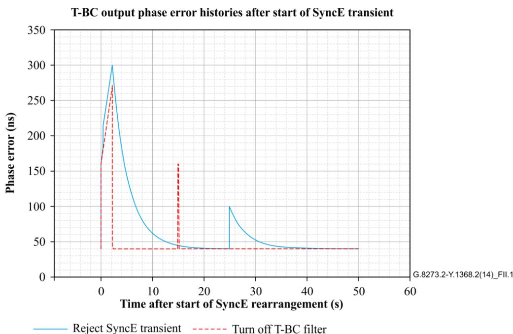
**Figure II.1 – T-BC output phase error histories for each of the two techniques, assuming SyncE/SDH transient starts at time zero**
