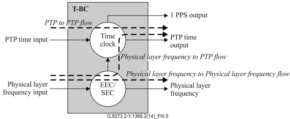
**Figure III.5 – Signal flows through a T-BC**
