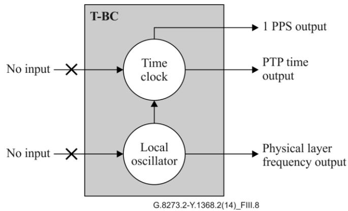
**Figure III.8 – Unassisted holdover**
