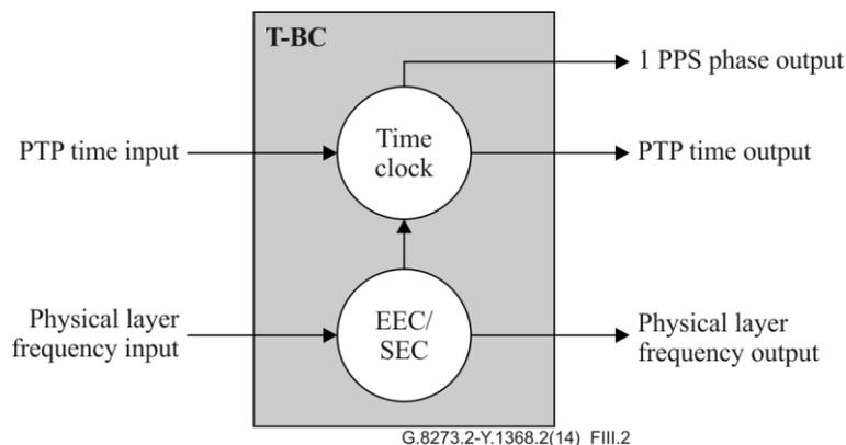
**Figure III.2 – Simplified model of T-BC showing clocks**
