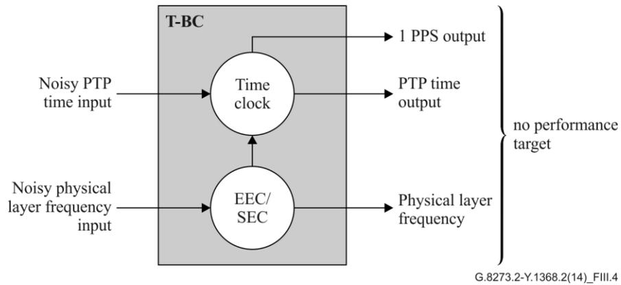
**Figure III.4 – Noise tolerance of a T-BC**
