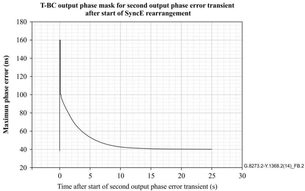
**Figure B.2 – Phase error limit for second output phase error transient after the start of the SyncE/SDH rearrangement**
