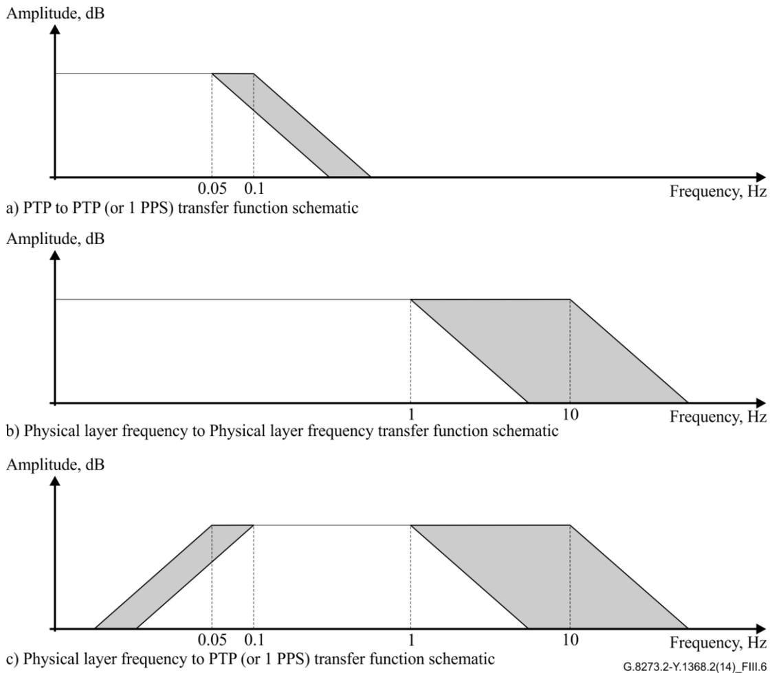
**Figure III.6 – Generalized transfer function schematics of a T-BC**
