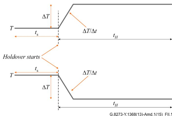
**Figure II.1 – Variable temperature profile for holdover testing**
