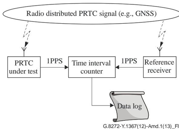
**Figure I.3 – Comparing time accuracy against a reference receiver**
