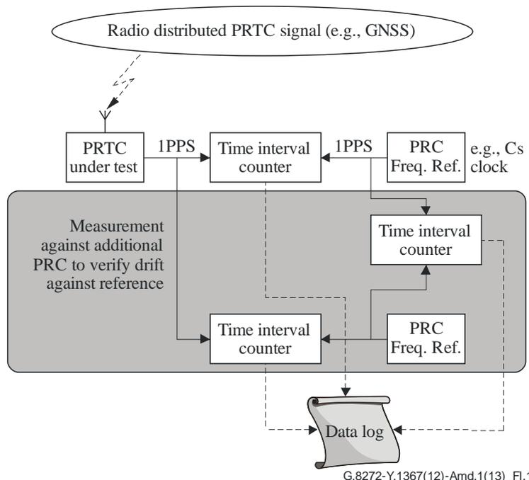
**Figure I.1 – Measuring phase wander of a PRTC**
