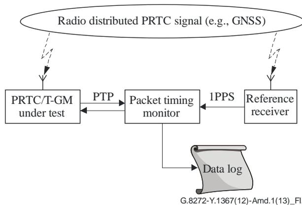
**Figure I.4 – Comparing time accuracy of a PRTC and T-GM against a reference receiver**
