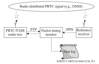
Figure I.4 – Comparing time accuracy of a PRTC and T-GM against a reference receiver
