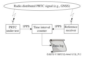
Figure I.3 – Comparing time accuracy against a reference receiver
