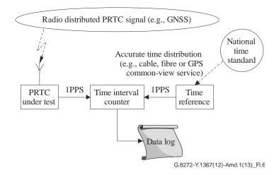
Figure I.6 – Measuring time accuracy against a national time standard
