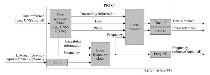
Figure II.1 – PRTC functional model
