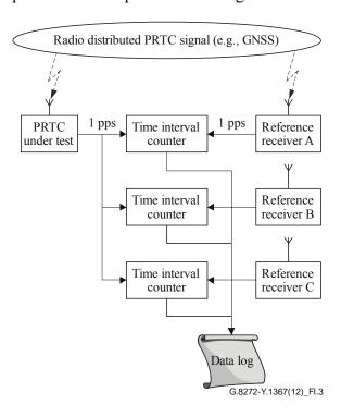
Figure I.3 – Comparing time accuracy against multiple reference receivers
