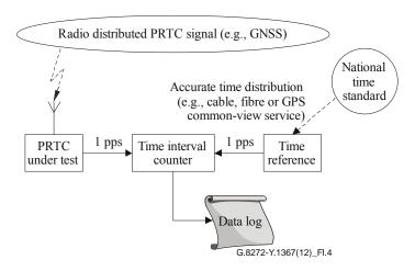
Figure I.4 – Measuring time accuracy against a national time standard
