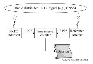
Figure I.2 – Comparing time accuracy against a reference receiver
