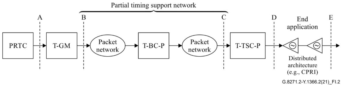
**Figure I.2 – Deployment case 1b (CPRI — common public radio interface)**
