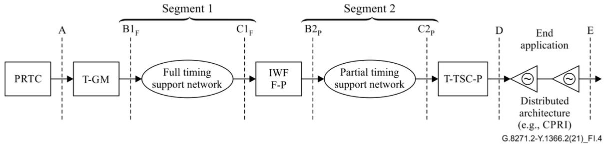
**Figure I.4 – Deployment case 2b (CPRI — common public radio interface)**
