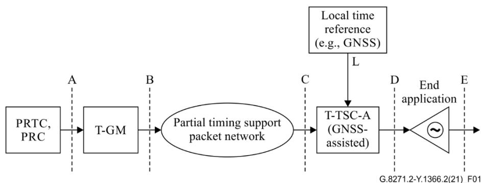
**Figure 1 – Reference model for network limits for APTS**
