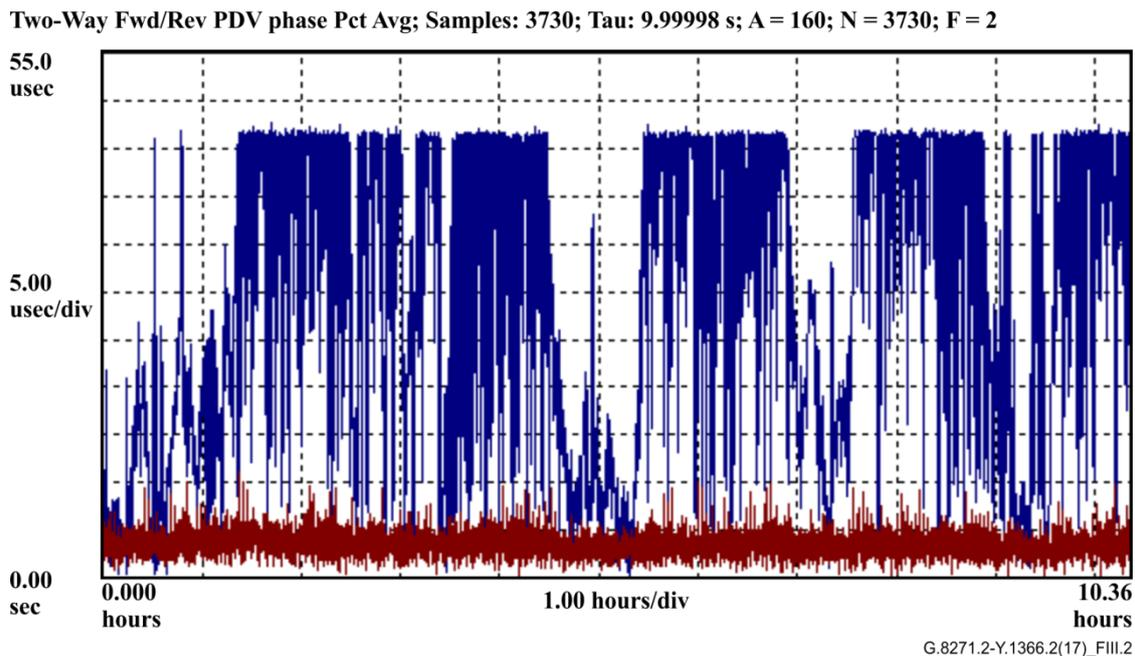
**Figure III.2 – Examples of forward and reverse packet sequences**
