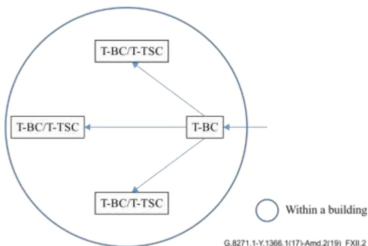
Figure XII.2 – Example of intra-station synchronization (co-located clocks)
