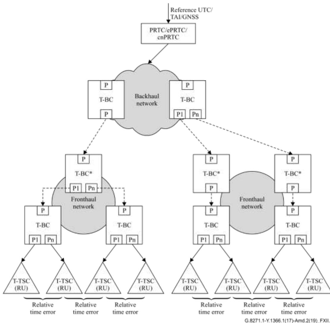
Case 1.1: Downstream T-BC located at the top of the fronthaul network connects to more than one T-BC through multiple ports.
