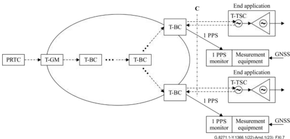
**Figure XI.7 – Maximum relative time error measurement in a field environment, with geographically separated measurement points and 1 PPS monitoring**
