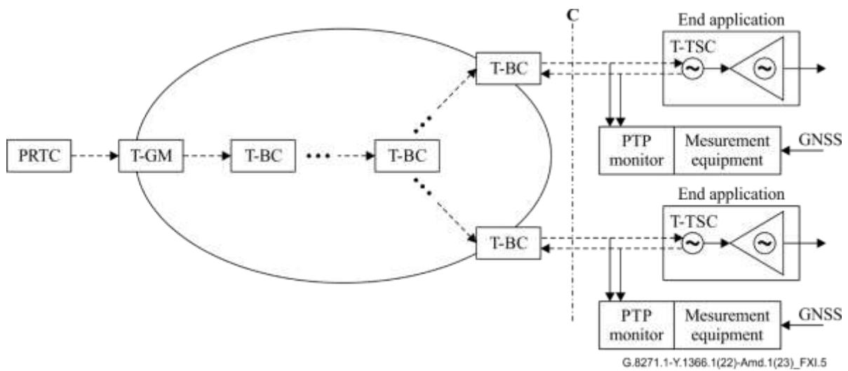
**Figure XI.5 – Maximum relative time error measurement in a field environment, with geographically separated measurement points and tapped monitoring**
