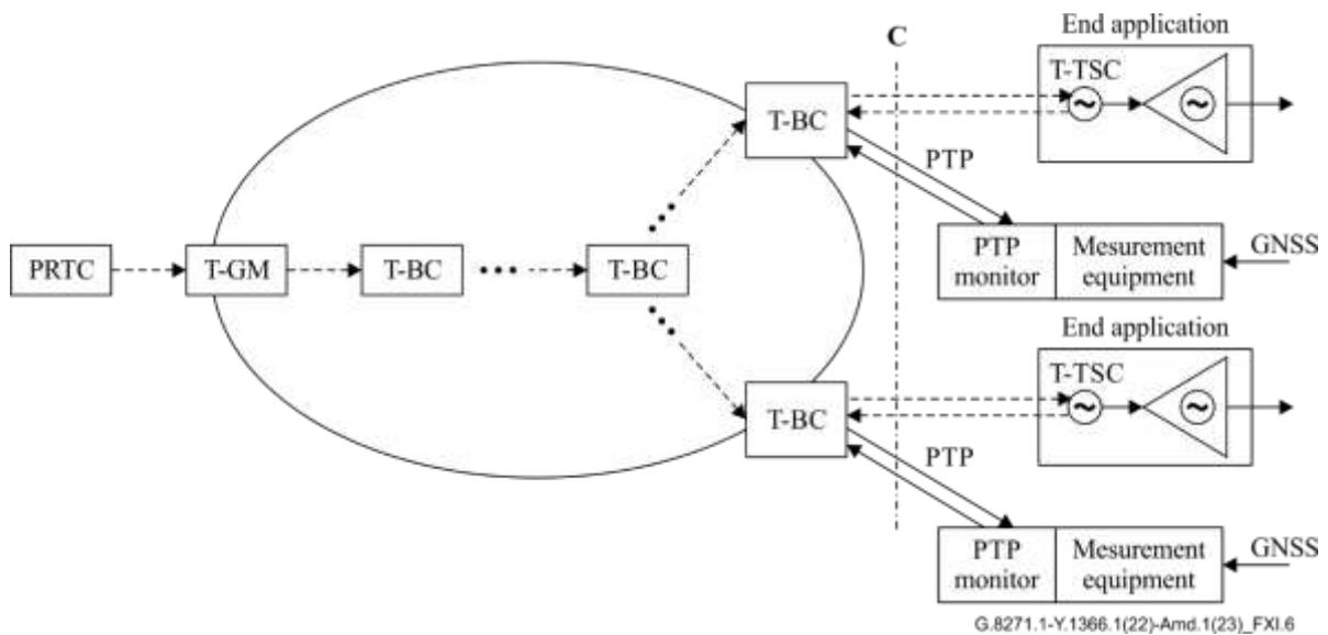
**Figure XI.6 – Maximum relative time error measurement in a field environment, with geographically separated measurement points and active monitoring**
