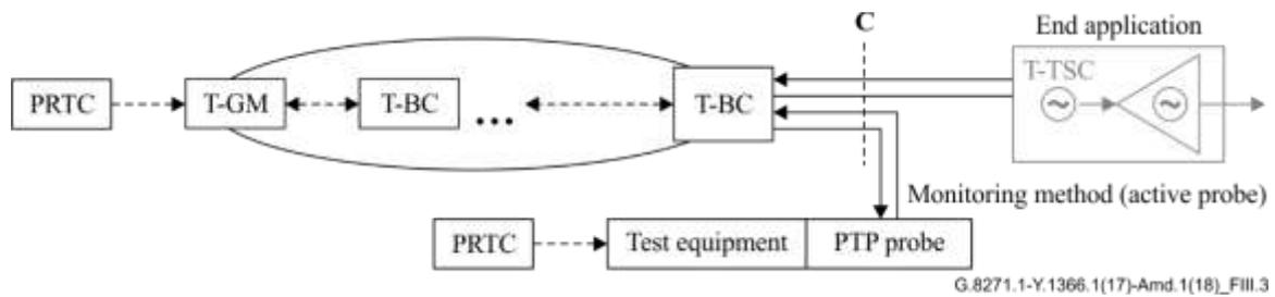
**Figure III.3 – Deployment case 1 network limits measurement, option c)**
