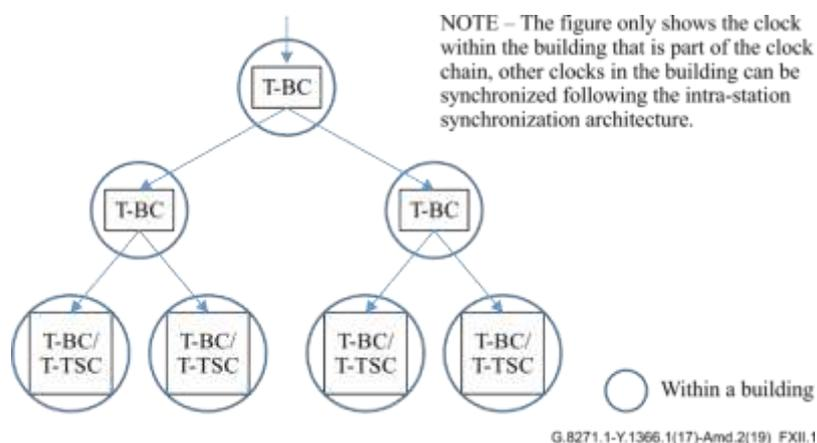
Figure XII.1 – Example of inter-station synchronization (non co-located clocks)
