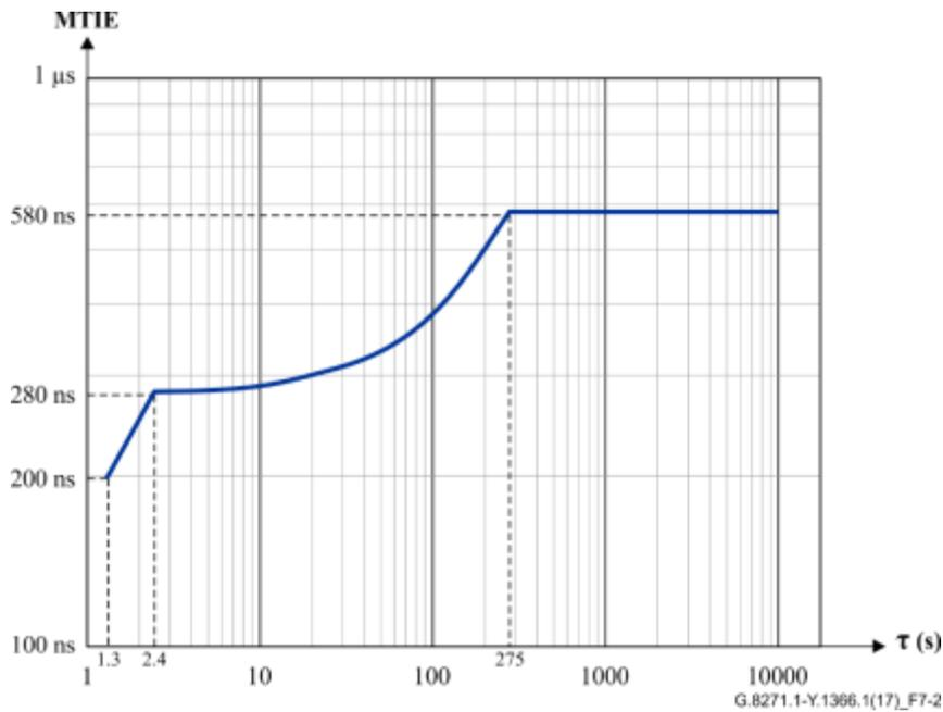
**Figure 7-2 – Dynamic time error network limit (MTIE)**
