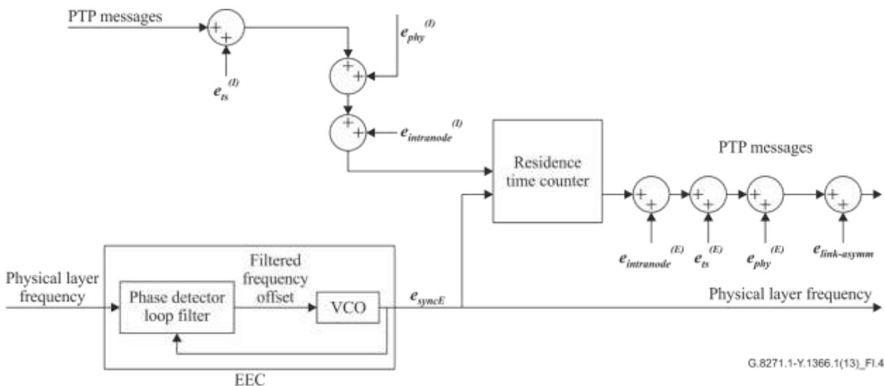
**Figure I.4 – Telecom end-to-end transparent clock model for simulating the transport of time using PTP with synchronous Ethernet assistance**
