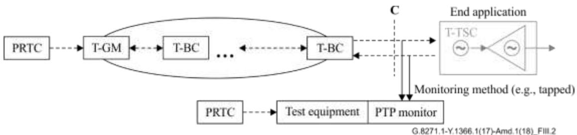
**Figure III.2 – Deployment case 1 network limits measurement, option b)**
