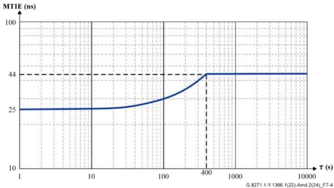
**Figure 7-4 – Dynamic time error network limit (MTIE)**
