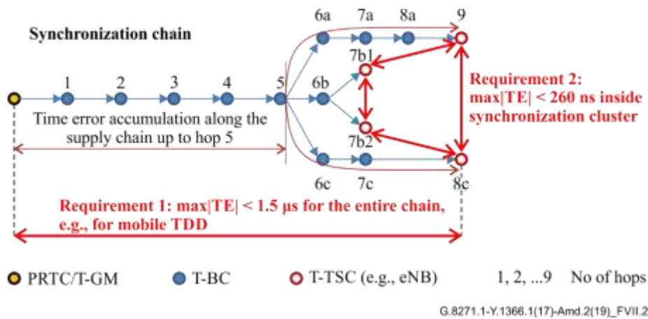
**Figure VII.2 – Illustration of relative time error monitoring example**
