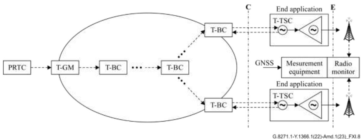
**Figure XI.8 – Maximum relative time error measurement in a field environment, monitoring the time alignment of the radio signals**
