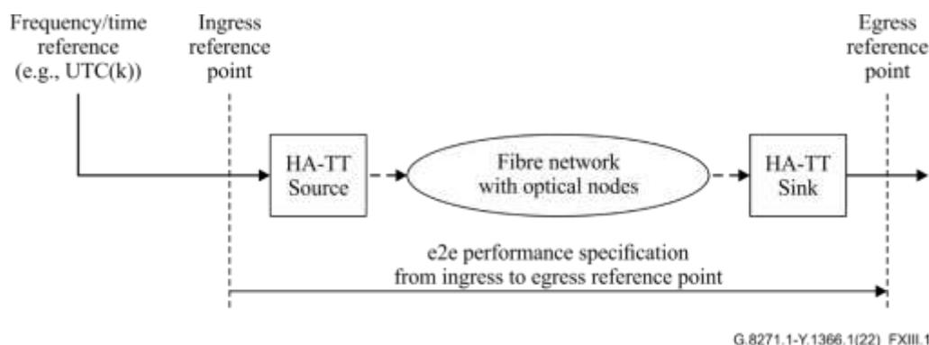
Figure XIII.1 – Reference chain for high-accuracy time transfer
