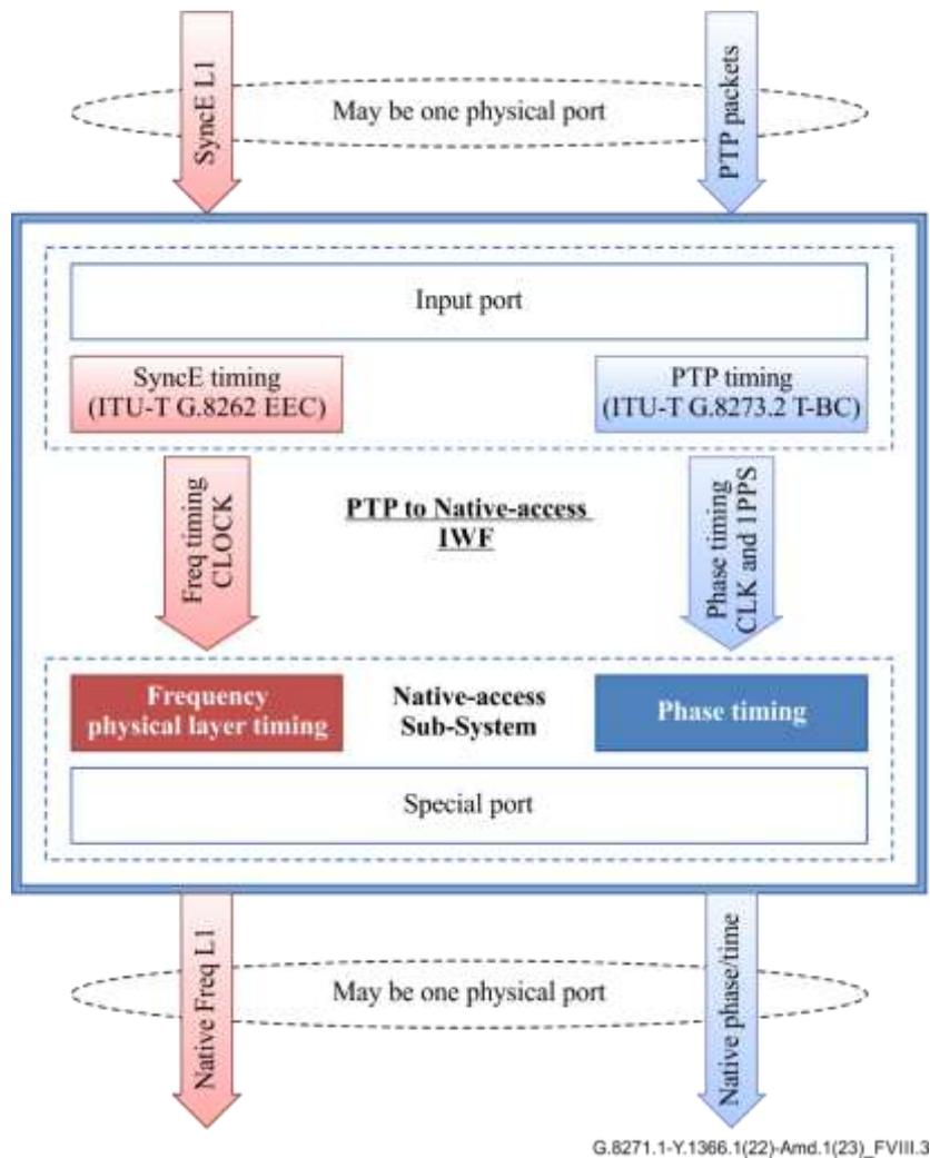
**Figure VIII.3 – Timing flow from PTP to native access medium (either direction)**
