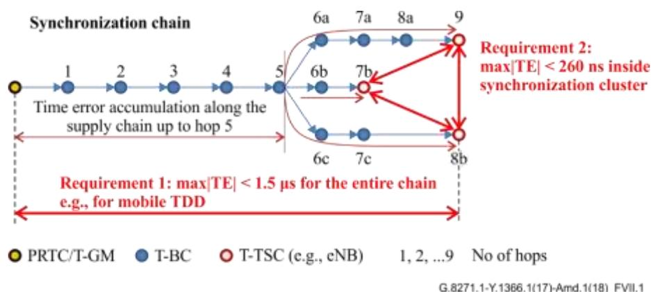
**Figure VII.1 – Illustration of relative time error**
