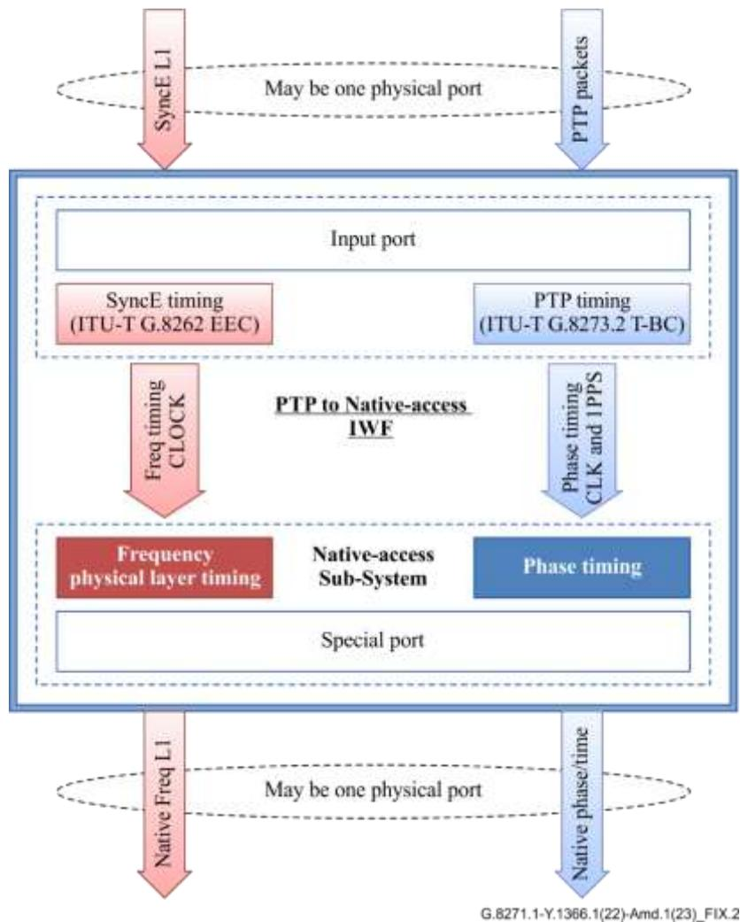
**Figure IX.2 – Timing flow from PTP to native access medium (downstream)**
