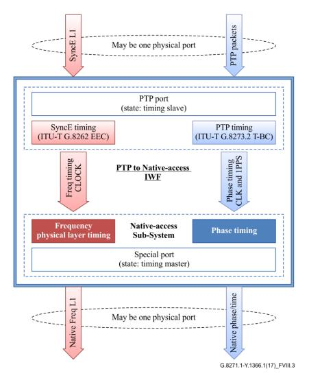
Figure VIII.3 – Timing flow from PTP to native access media (either direction)
