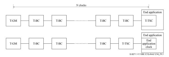
Figure II.1 – HRM-1 without physical layer frequency support
