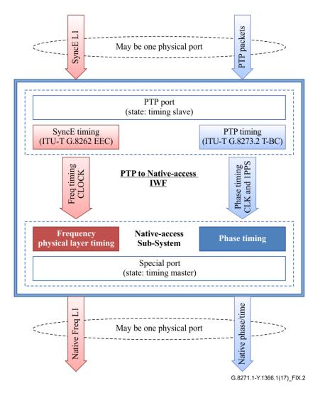
Figure IX.2 – Timing flow from PTP to native access media (downstream)
