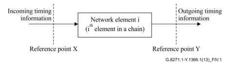
**Figure IV.1 – Accumulation of time error**
