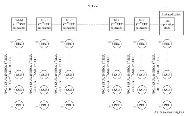
Figure II.5 – HRM-3 with physical layer frequency support – non-congruent scenario, deployment case 2
