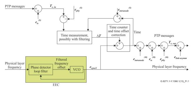
Figure I.1 – Telecom boundary clock model for simulating the transport of time using PTP with synchronous Ethernet assistance
