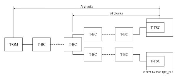
Figure II.6 – HRM-4 for cluster based synchronization without physical layer frequency support
