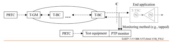
Figure III.2 – Deployment case 1 network limits measurement, option b)
