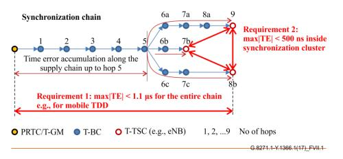
Figure VII.1 – Illustration of relative time error
