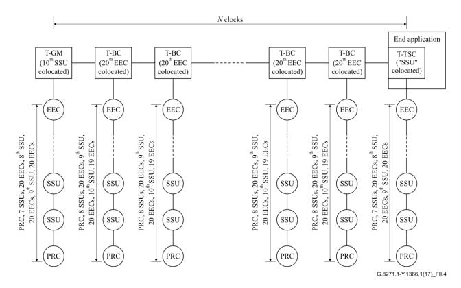
Figure II.4 – HRM-3 with physical layer frequency support – non-congruent scenario, deployment case 1
