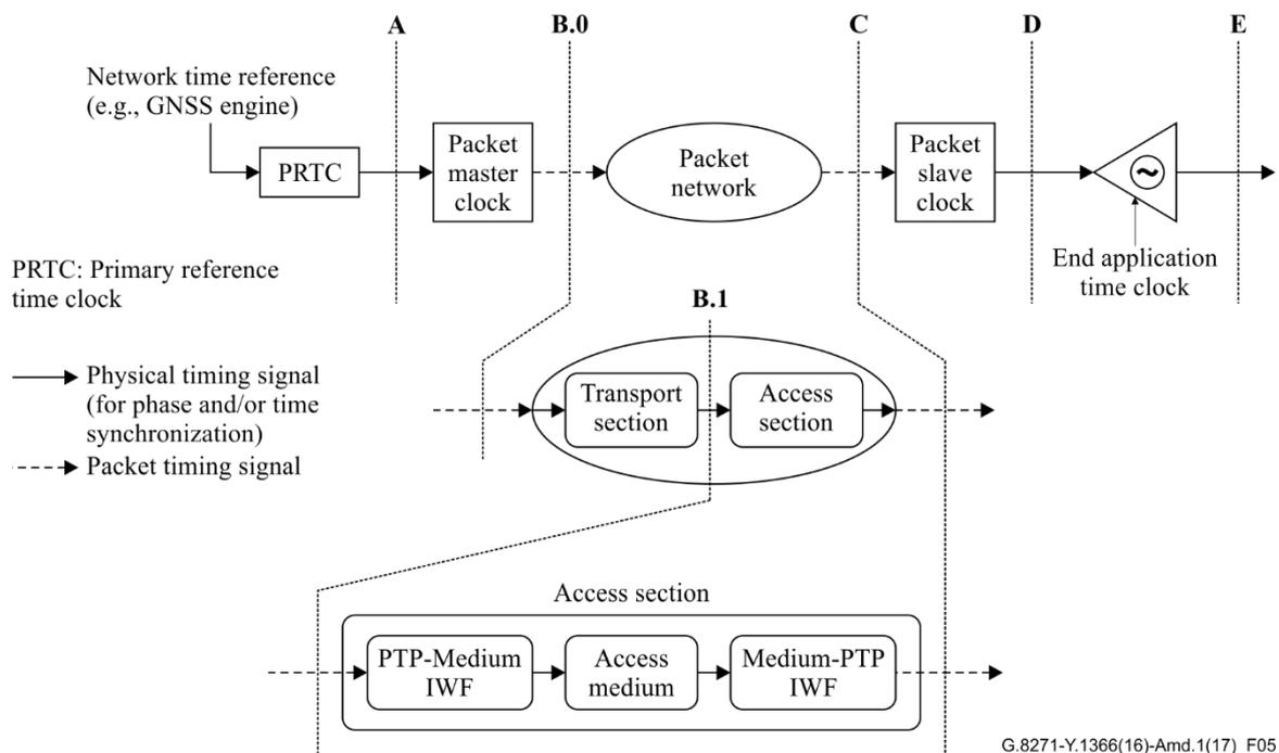
**Figure 5 – Network reference model with access section**
