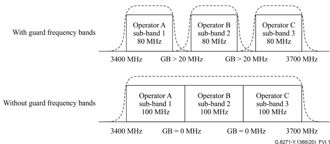
**Figure VI.1 – Examples of frequency allocation for TDD systems with and without guard frequency bands**
