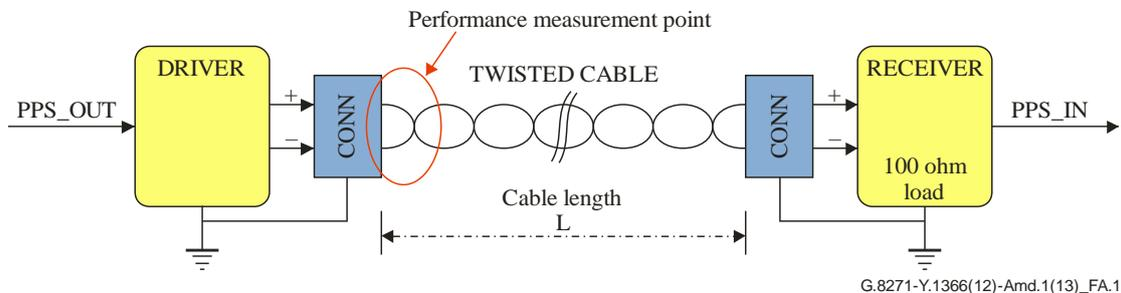
**Figure A.1 – Balanced 1PPS V.11 interface**
