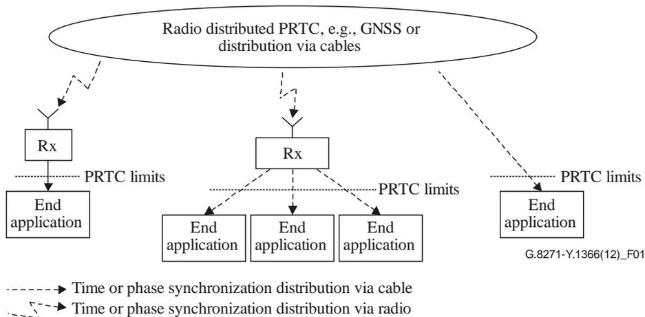
**Figure 1 – Example of a distributed PRTC synchronization network**
