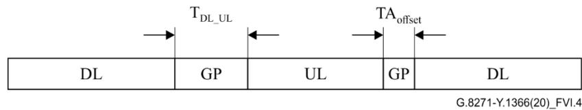
**Figure VI.4 – Signal frame format of TDD systems**
