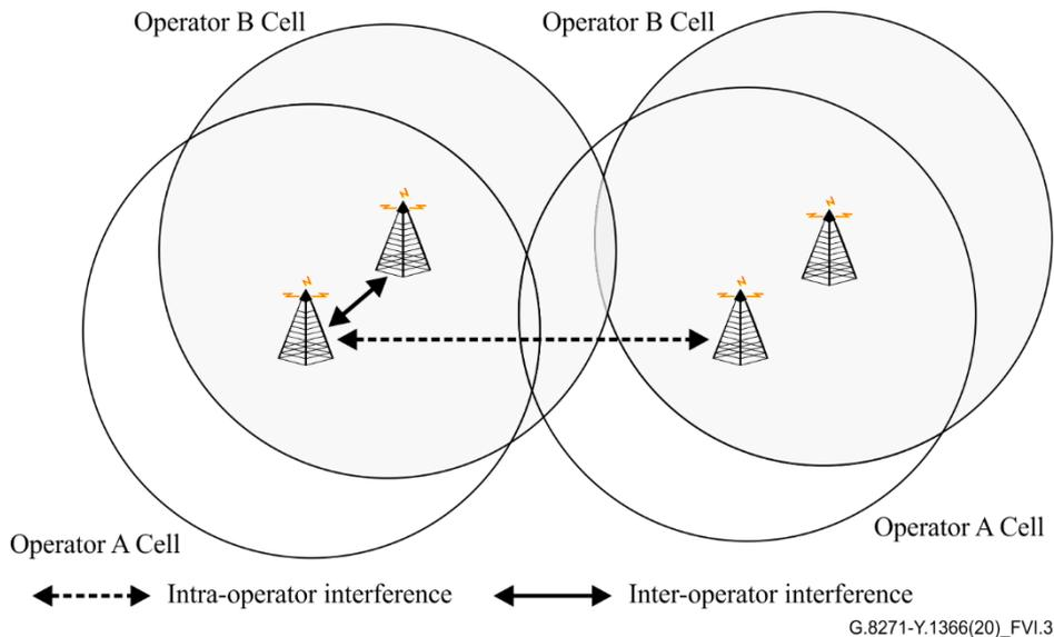
**Figure VI.3 – Relationship between intra- and inter-operator interference**
