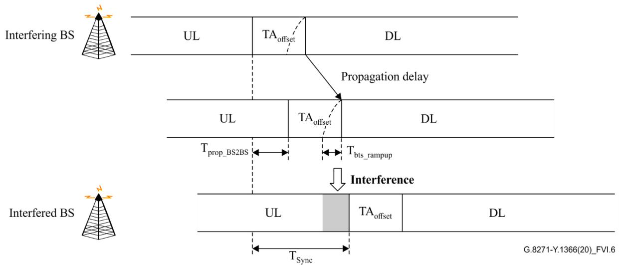
**Figure VI.6 – BS to BS interference at UL to DL switching point**
