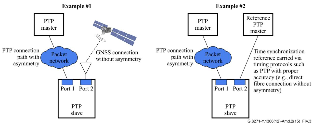
**Figure IV.3 – PTP slave evaluating PTP connection asymmetry**
