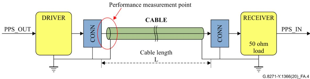
**Figure A.4 – Unbalanced 1PPS 50 Ω measurement interface**
