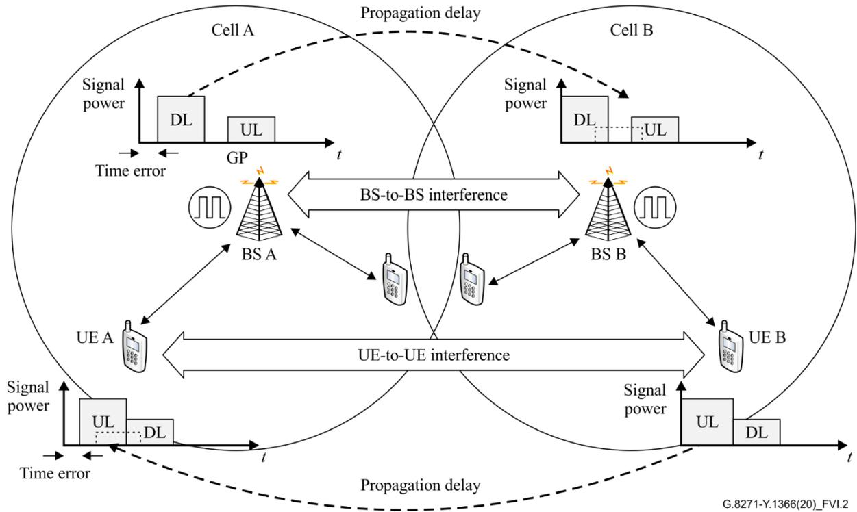
**Figure VI.2 – Overview of interference patterns in TDD systems**
